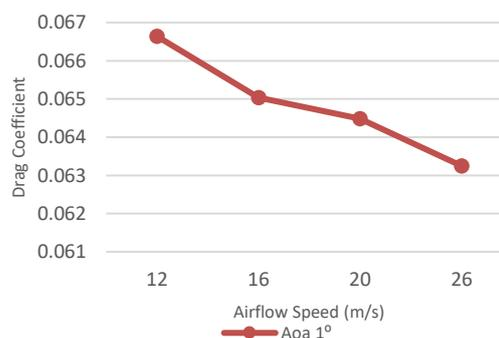
Fig. 12. The effect of airflow on  $C_D$
