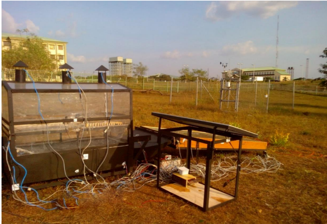
Fig. 9. Positioning of the sensors at different locations on a solar drying system for data capturing [21-25]
