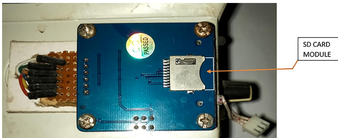
Fig. 3. Data logging device indicating the SD card module
