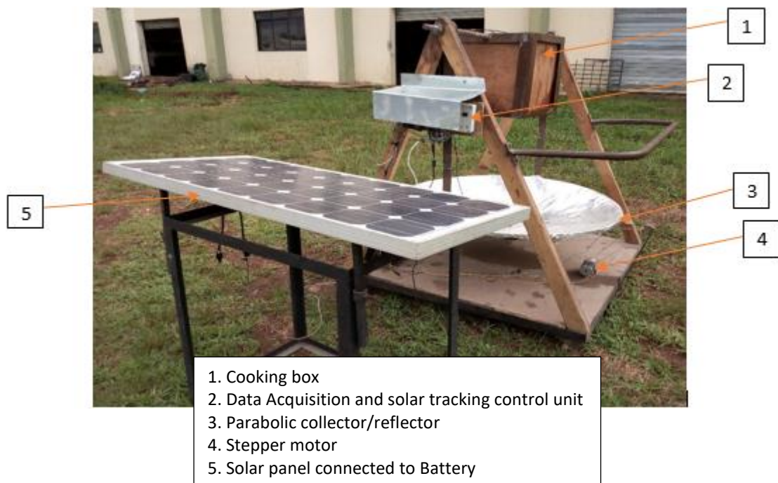
Fig. 10. Application on solar cooking system [26]
