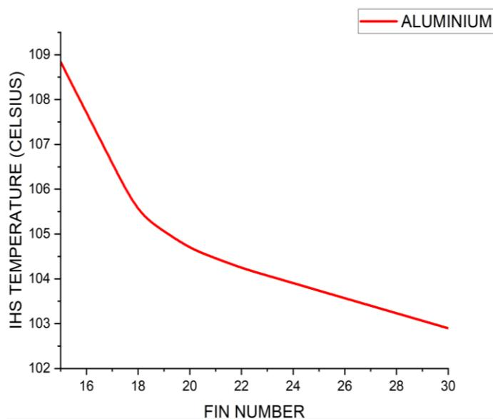
Fig. 4. Fin number optimization for Aluminium heatsink
