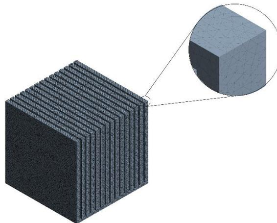
**Fig. 1.** Heatsink with Tetrahedral meshing
