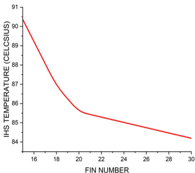
Fig. 5. Fin number optimization for Copper heatsink
