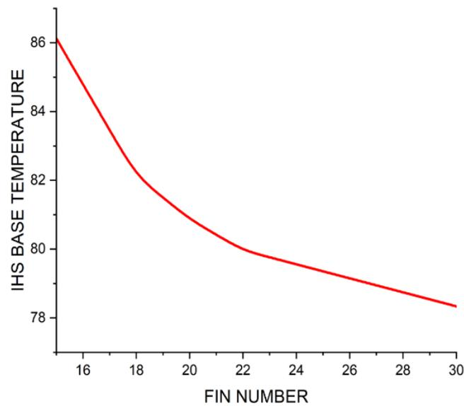
**Fig. 6.** Fin number optimization for Silicon Carbide heatsink
