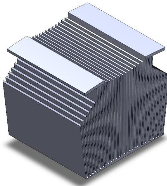
**Fig. 7.** Optimal design after topology optimization
