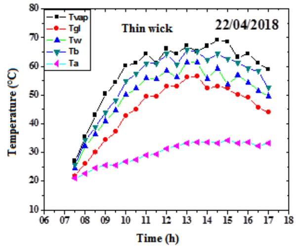
Fig. 6. Variation of solar still components temperatures with thin wick
