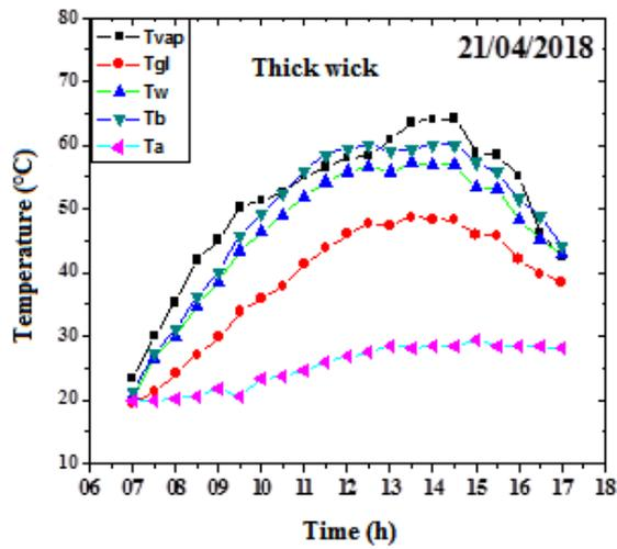
Fig. 5. Variation of solar still components temperatures with thick wick
