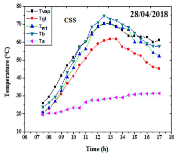
Fig. 8. Variation of conventional solar still components temperatures
