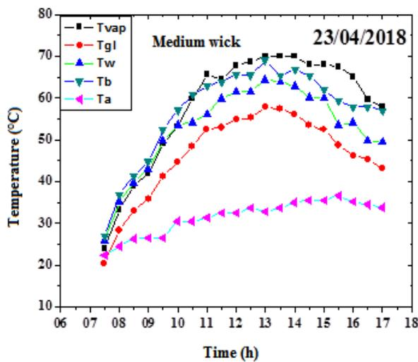
Fig. 7. Variation of solar still components temperatures with medium wick
