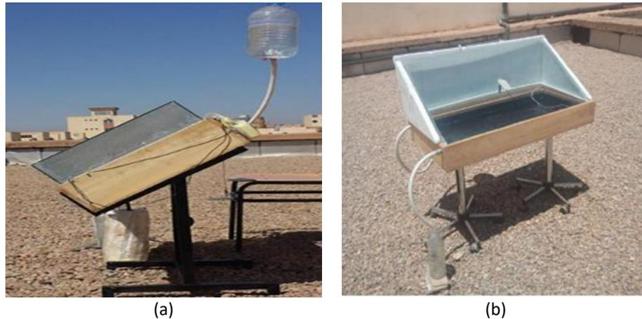
**Fig. 2.** A photograph of the test-rig setup (a) inclined wick solar still (b) conventional solar still
