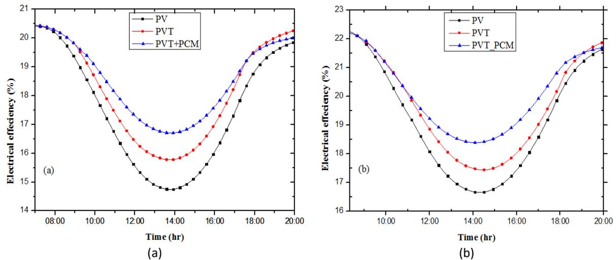
**Fig. 6.** Fluctuation in the PV panel's electrical efficiency over time for different systems during the 4th of August, 2022 (a), and the 4th of January, 2023 (b)
