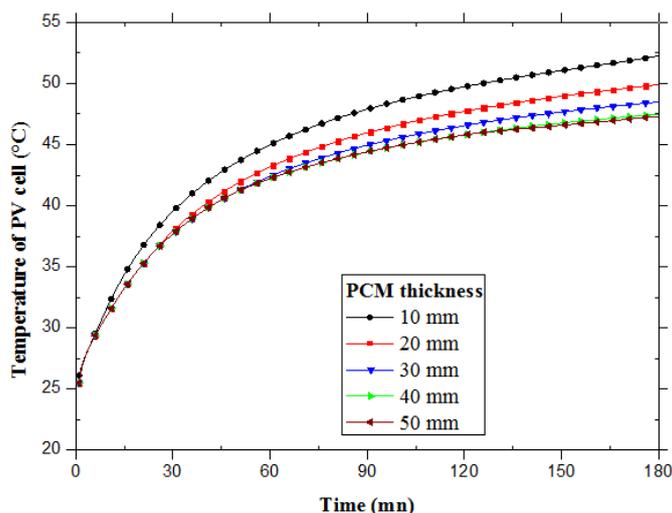
**Fig. 7.** The impact of PCM layer thickness on PV temperature compared to a conventional PV module without PCM
