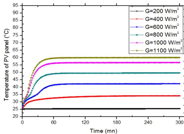
**Fig. 9.** The effect of irradiation on the PV panel temperature in the PV/T-PCM system
