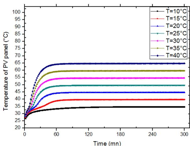
**Fig. 8.** The impact of the ambient temperature on the PV panel temperature in the PV/T-PCM system
