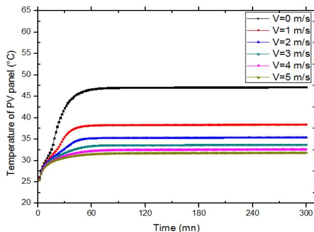
**Fig. 10.** The effect of the wind speed on the PV panel temperature in the PV/T-PCM system
