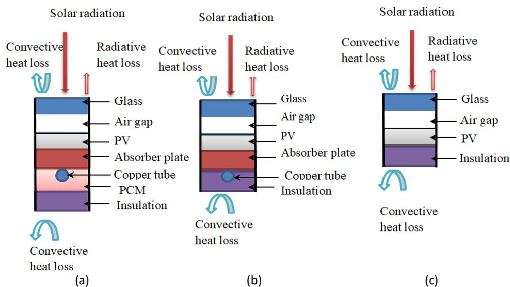
**Fig. 1.** The design of the front view of the (a) PV/T-PCM, (b) PV/T system, and (c) standalone PV system
