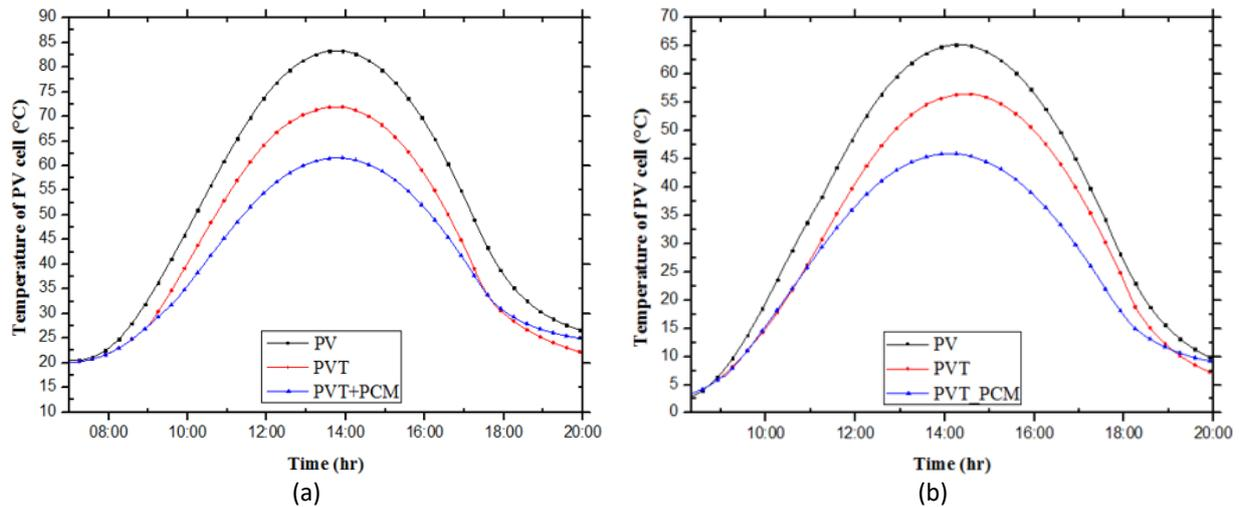
**Fig. 5.** Variation in the PV panel's temperature over time in different systems during (a) the 4th of August, 2022 and (b) the 4th of January, 2023
