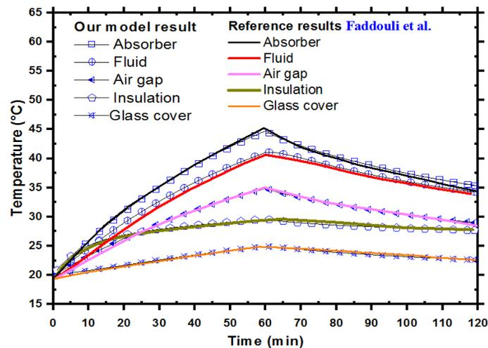
**Fig. 2.** The expected temperatures compared with that achieved by Faddouli *et al.*, [33]
