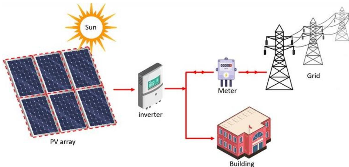
**Fig. 1.** Schematic of the proposed rooftop grid-connected system
