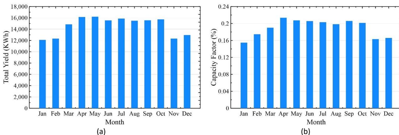
**Fig. 12.** Monthly (a) energy yield and (b) Capacity factor of the considered PV system
