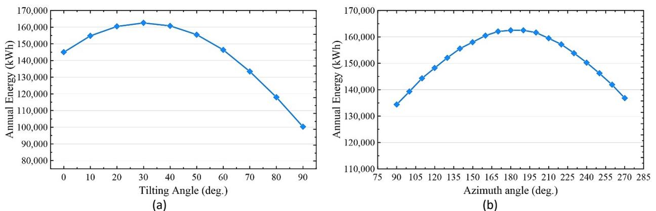
Fig. 8. The effect of (a) Tilt angle (b) Azimuth angle on the production of 75 kW PV array
