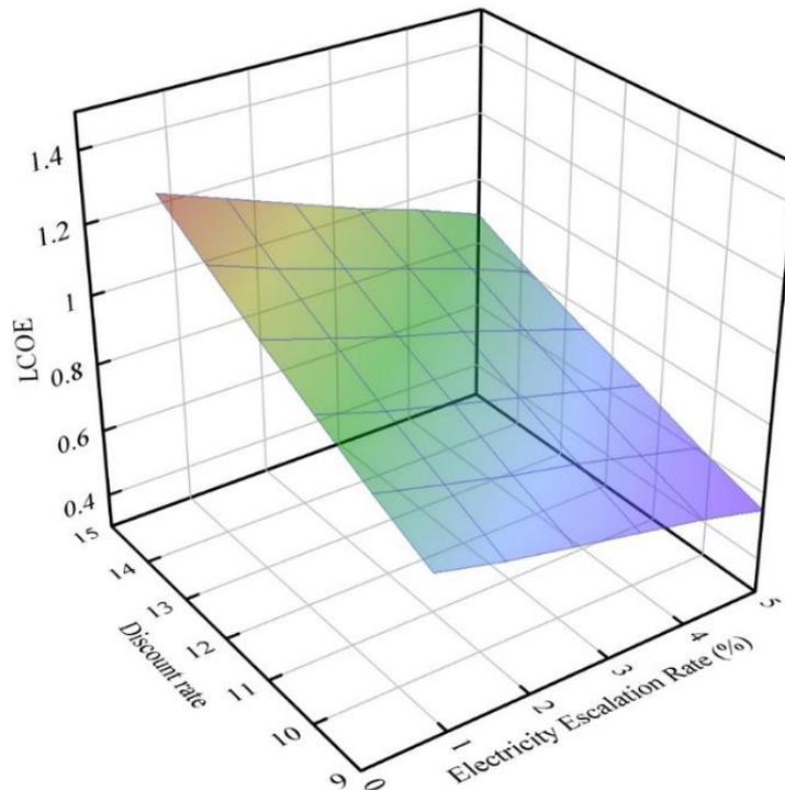
**Fig. 16.** Sensitivity of LCOE to changes in the discount rate and the electricity escalation rate
