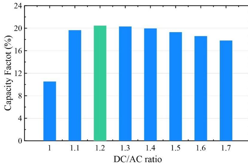
**Fig. 10.** DC/AC ratio effect on the capacity factor % of kW<sub>AC</sub> PV system
