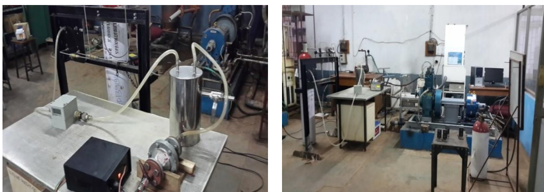
Fig. 3. Gas supply arrangement with dual fuel engine test rig
