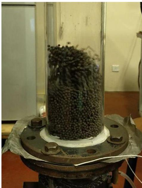
**Fig. 16.** The swirling condition of the piper nigrum using a 67° angle distributor in fluidized bed dryer
