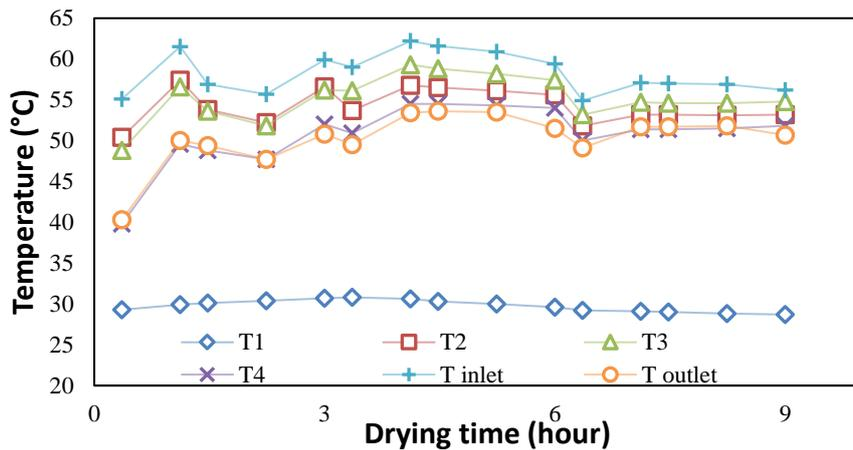
**Fig. 12.** The temperature vs drying time taken at high temperature using perforated distributor
