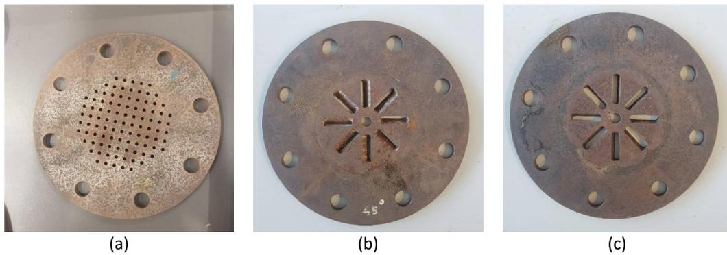
**Fig. 5.** The photograph of the different inclination angle distributor, (a) perforated distributor, (b) 45° distributor, (c) 67° distributor
