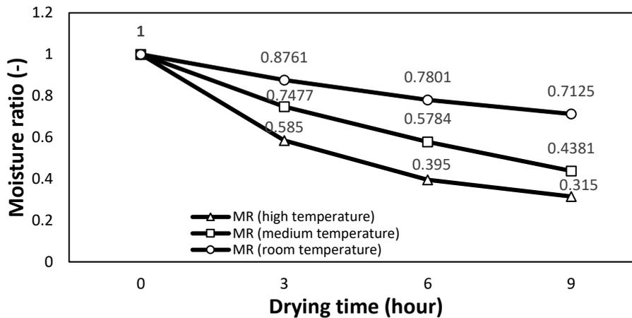
**Fig. 11.** The graph of the drying at three different temperature using perforated distributor
