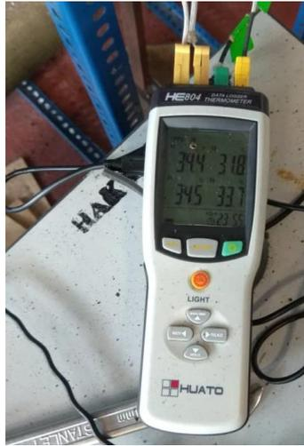
**Fig. 3.** The HUATO HE804 temperature data logger for temperature recording
