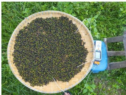
**Fig. 1.** The conventional sun drying set up with the data logger
