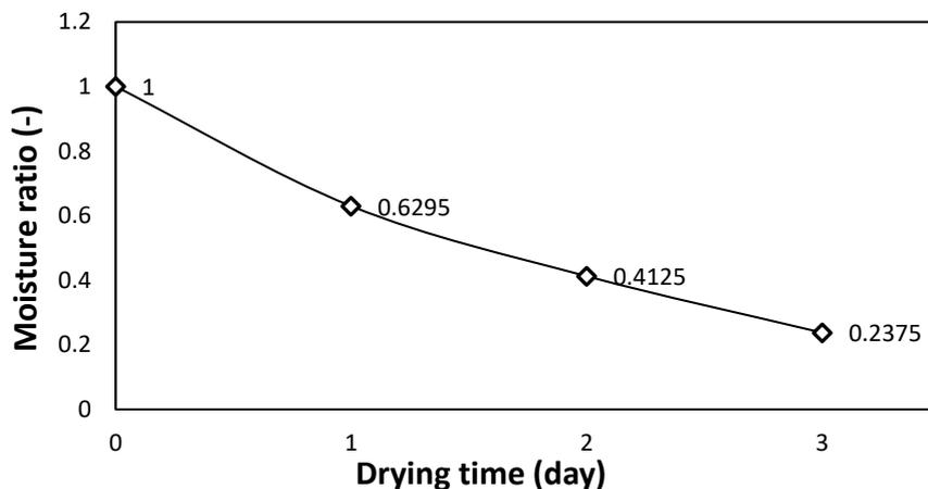
**Fig. 7.** Graph of the moisture ratio of conventional sun drying vs time taken for drying
