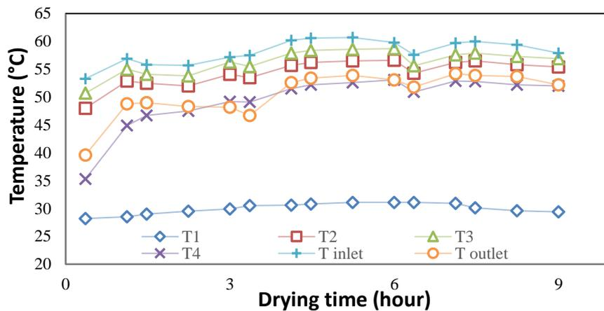
**Fig. 18.** The high temperature vs drying time at high temperature using 67° angle distributor
