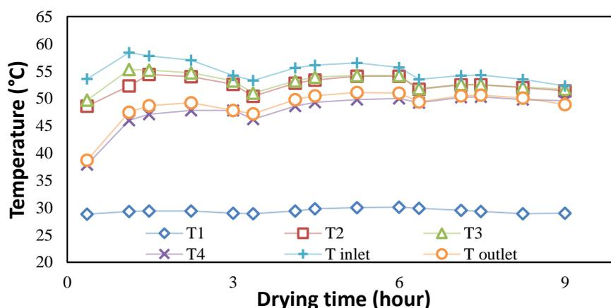
**Fig. 15.** The high temperature vs drying time at high temperature using 45° angle distributor
