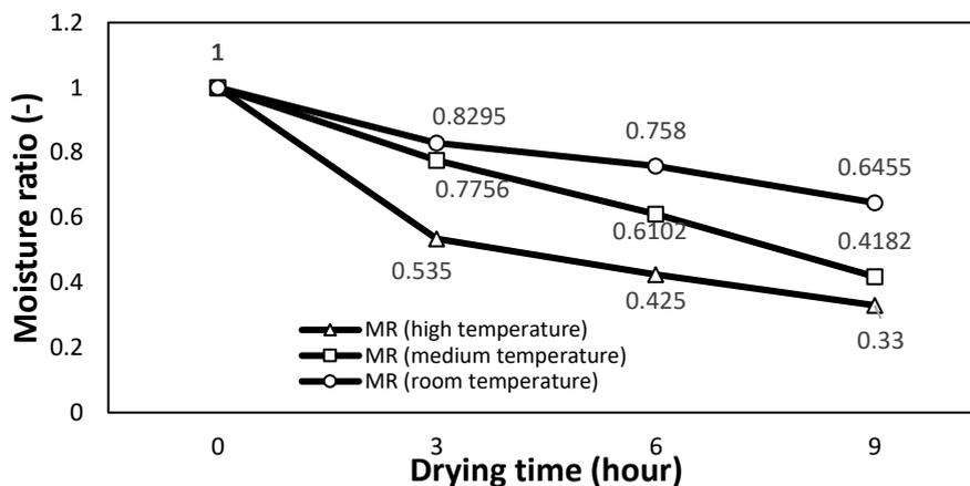
**Fig. 17.** The graph of the drying at three different temperatures using 67° angle distributor
