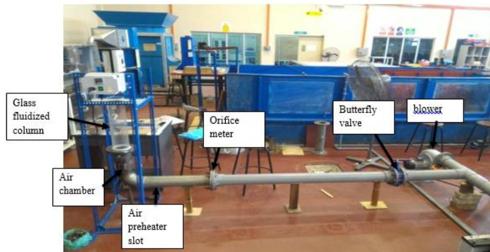
**Fig. 2.** The swirling fluidized bed dryer setup
