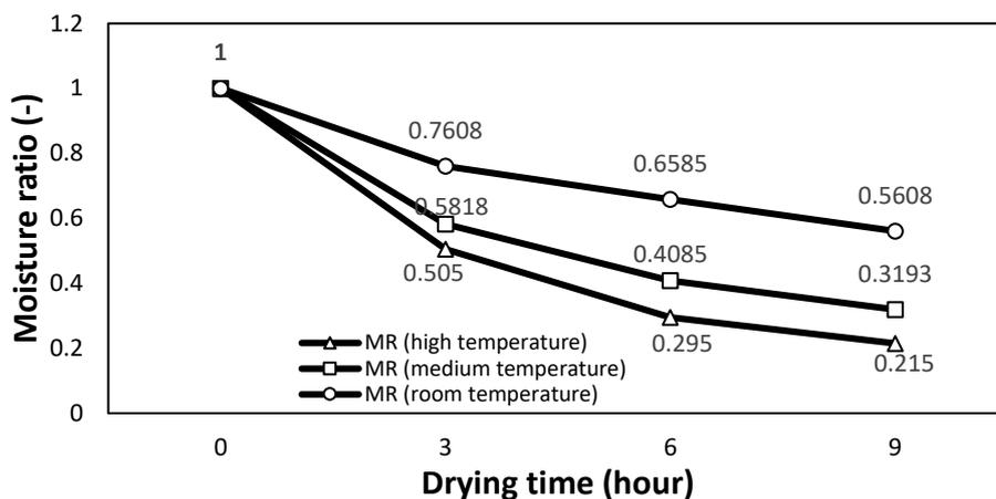
**Fig. 14.** The graph of the drying at three different temperatures using 45° angle distributor
