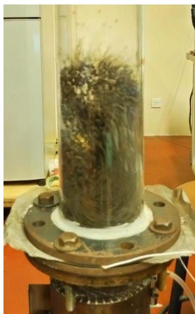
**Fig. 13.** The swirling pattern of the piper nigrum during the drying process using a 45° angle distributor
