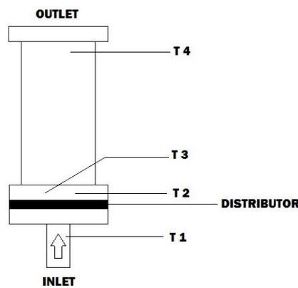
**Fig. 4.** Schematic diagram of the position of the thermocouple at fluidized bed dryer
