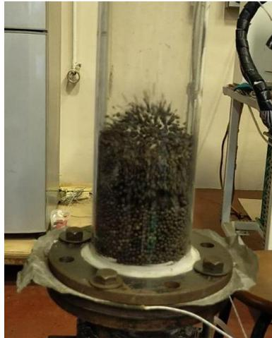
**Fig. 10.** The swirling pattern of piper nigrum using a perforated distributor
