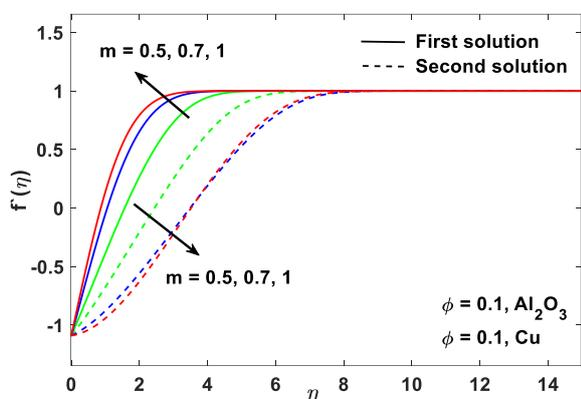
**Fig. 4.** Velocity profiles  $f'(\eta)$  for different values of  $m$  when  $\varphi_1 = \varphi_2 = 0.1$  and  $\lambda = -1.09$  for  $\text{Al}_2\text{O}_3$ - Cu/water hybrid nanofluid
