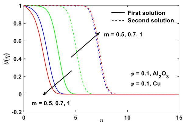
**Fig. 5.** Temperature profiles  $\theta(\eta)$  for different values of  $m$  when  $\varphi_1 = \varphi_2 = 0.1$  and  $\lambda = -1.09$  for  $\text{Al}_2\text{O}_3$ - Cu/water hybrid nanofluid
