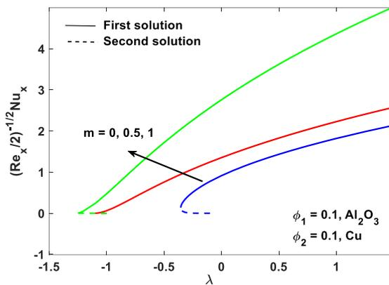
**Fig. 3.** Variation of local Nusselt number with  $\lambda$  for different values of  $m$  when  $\varphi_1 = \varphi_2 = 0.1$  for  $\text{Al}_2\text{O}_3$ - Cu/water hybrid nanofluid
