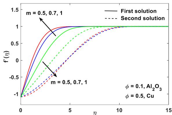
**Fig. 6.** Velocity profiles  $f'(\eta)$  for different values of  $m$  when  $\varphi_1 = 0.1$ ,  $\varphi_2 = 0.5$  and  $\lambda = -1.09$  for  $\text{Al}_2\text{O}_3$ - Cu/water hybrid nanofluid
