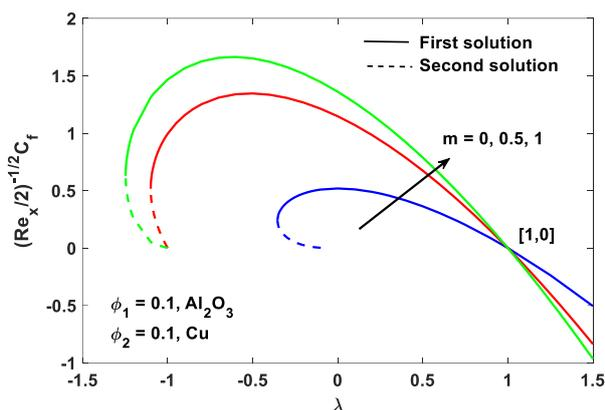
**Fig. 2.** Variation of skin friction coefficient with  $\lambda$  for different values of  $m$  when  $\varphi_1 = \varphi_2 = 0.1$  for  $\text{Al}_2\text{O}_3$ - Cu/water hybrid nanofluid
