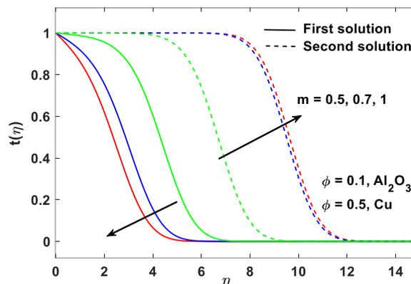
**Fig. 7.** Temperature profiles  $\theta(\eta)$  for different values of  $m$  when  $\varphi_1 = 0.1$ ,  $\varphi_2 = 0.5$  and  $\lambda = -1.09$  for  $\text{Al}_2\text{O}_3$ - Cu/water hybrid nanofluid
