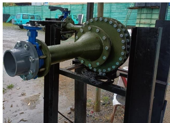
Fig. 2. Fabricated turbine body assembled on steel structure
