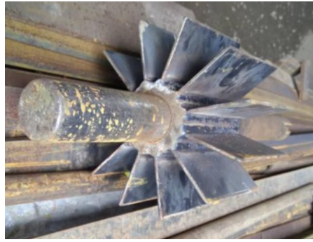
Fig. 4. Runner blade and 2" shaft mated using keyway locking system
