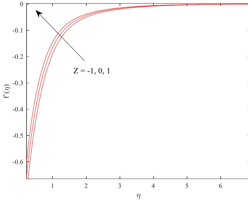
**Fig. 12.** Velocity profiles  $f'(\eta)$  vs  $\eta$  for various values of  $Z$  where  $\varepsilon = -1$ ,  $S = 2.4$ ,  $\lambda = 1.5$ ,  $\gamma = 0.1$ ,  $Pr = 10$ ,  $\phi_1 = 0.01$  and  $\phi_2 = 0.02$
