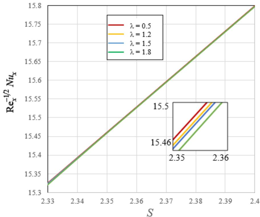
**Fig. 3.**  $Re_x^{-1/2} Nu_x$  vs  $S$  for various values of  $\lambda$  where  $\varepsilon = -1$ ,  $\gamma = 0.1$ ,  $Pr = 10$  and  $Z = -0.5$
