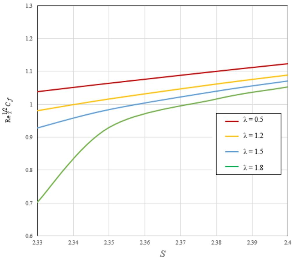
Fig. 2.  $Re_x^{1/2} C_f$  vs  $S$  for various values of  $\lambda$  where  $\varepsilon = -1$ ,  $\gamma = 0.1$ ,  $Pr = 10$  and  $Z = -0.5$
