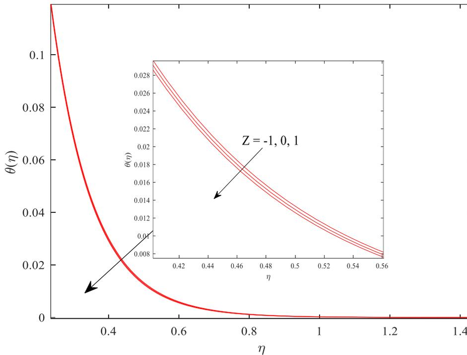
**Fig. 13.** Temperature profiles  $\theta(\eta)$  vs  $\eta$  for various values of  $Z$  where  $\varepsilon = -1$ ,  $S = 2.4$ ,  $\lambda = 1.5$ ,  $\gamma = 0.1$ ,  $Pr = 10$ ,  $\phi_1 = 0.01$  and  $\phi_2 = 0.02$
