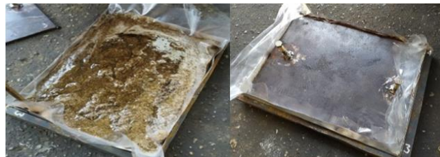
Fig. 3. Composite wall slabs before printing
