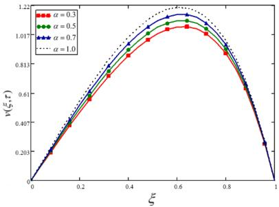
**Fig. 1.** Variations in velocity profile against  $\xi$  if  $h(\tau) = 0$  for different values of  $\alpha$  when  $\tau = 2$ ,  $\gamma_B = 0.5$ , Gm = 15, Sc = 5 and M = 1.5
