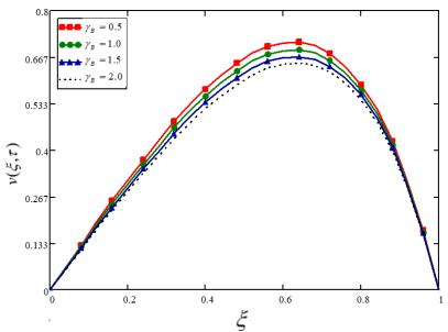
**Fig. 2.** Variations in velocity profile against  $\xi$  if  $h(\tau) = 0$  for different values of  $\gamma_B$  when  $\tau = 2$ ,  $\alpha = 0.5$ , Gm = 15, Sc = 5 and M = 1.5
