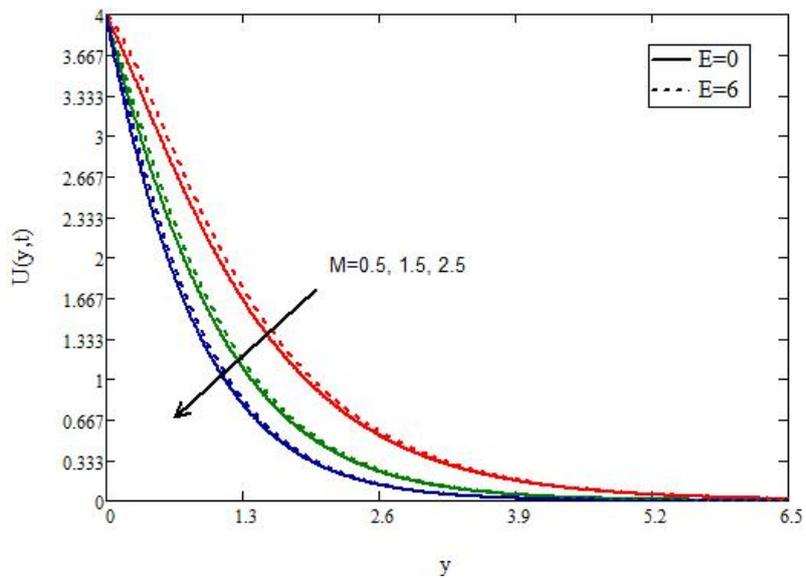
**Fig. 6.** Impact of  $M$  on velocity profile with and without presence of Riga Plate
