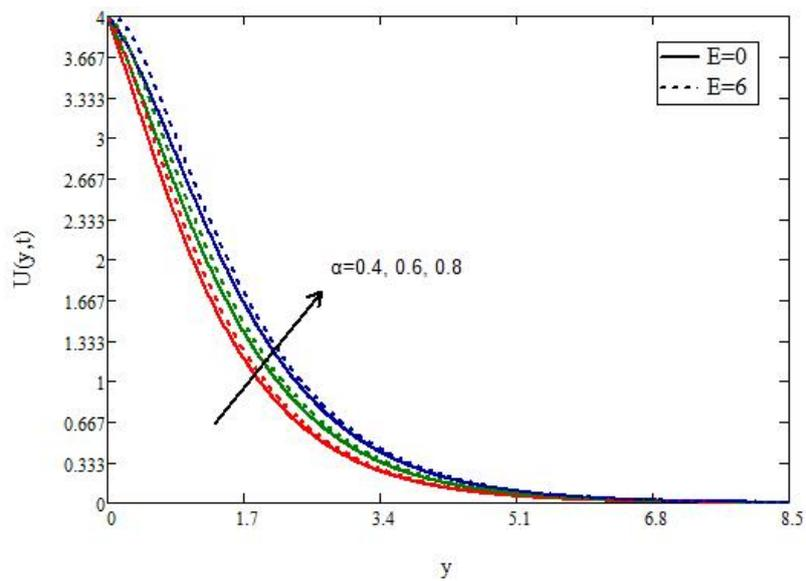
**Fig. 3.** Impact of  $\alpha$  on velocity profile with and without presence of Riga Plate
