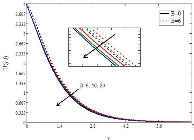
**Fig. 4.** Impact of  $\beta$  on velocity profile with and without presence of Riga Plate
