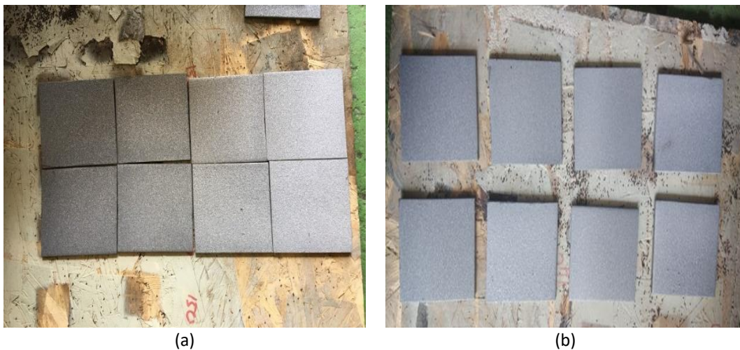
Fig. 2. Substrate materials (a) before and (b) after sandblasting
