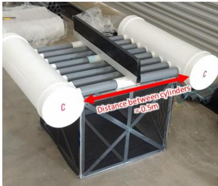
**Fig. 1.** Double cylindrical floating breakwater used in this study
