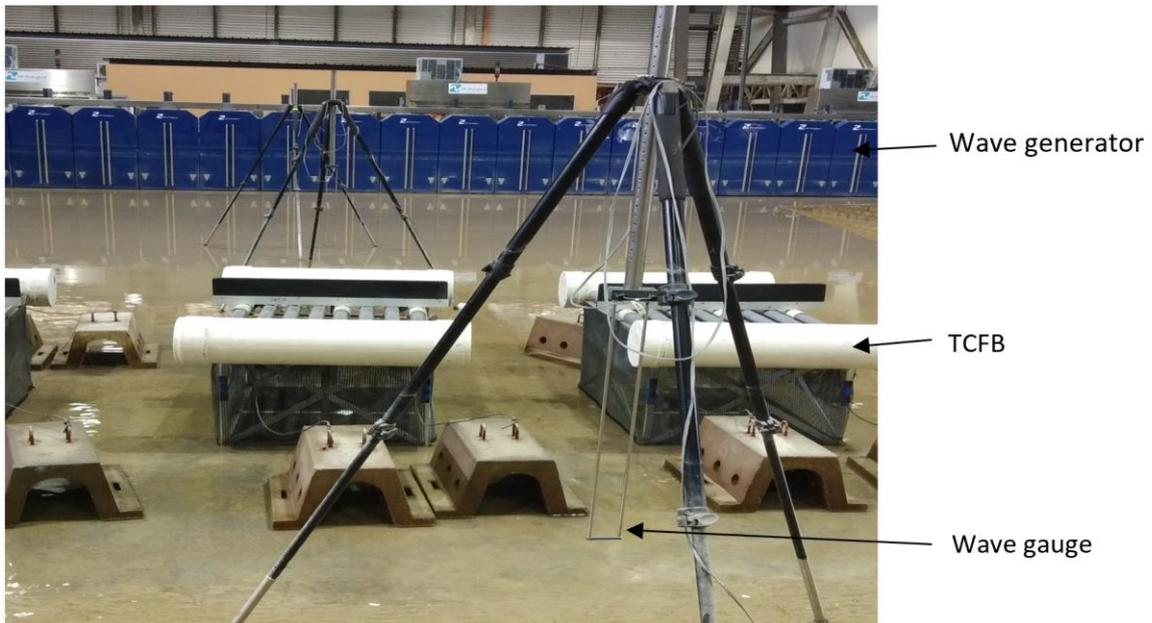
**Fig. 2.** The physical setup of the three units of twin cylindrical floating breakwater, showing pairs of floating cylinders to form a floating breakwater and the position of wave generator and wave gauges
