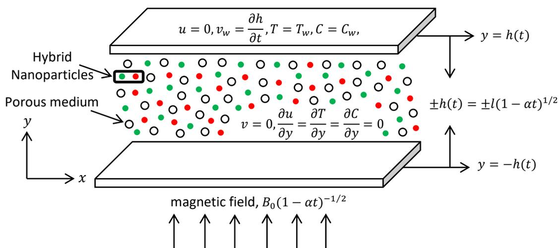
Fig 1. Geometry model of squeeze flow of hybrid nanofluid
