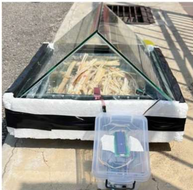
Fig. 8. The experiment of Bagasse inside Triangular-Prism Solar Still
