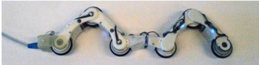
Fig. 5. Robot design with Ethernet as the tether
