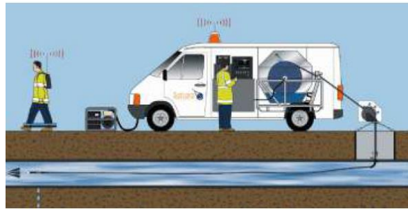
Fig. 2. Sahara Pipeline Inspection
