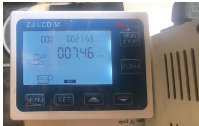
Fig. 23. Flowmeter reading during stable flow at 150V voltage supply
