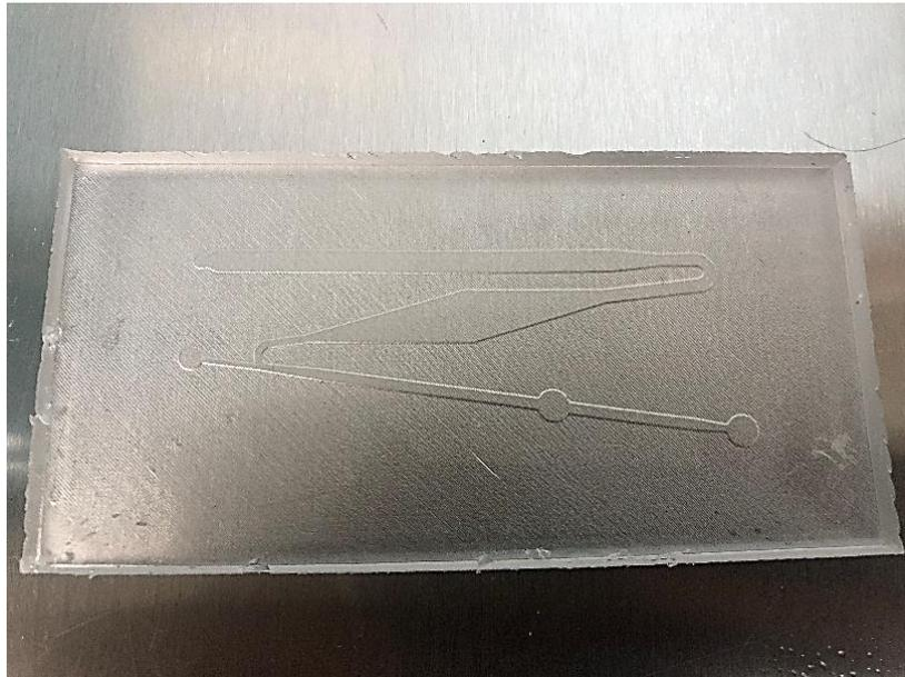
**Fig. 3.** Cured PDMS replica mold fabricated using 3D printed mold
