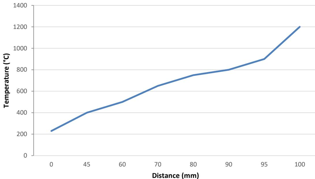
**Fig. 3.** Heat distribution along the plate
