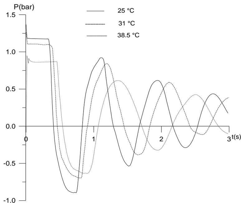
**Fig. 5.** Effect of the viscoelasticity with temperature
