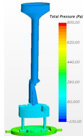
Fig. 5. Pressure profiles in the airway of the E-cigarette
