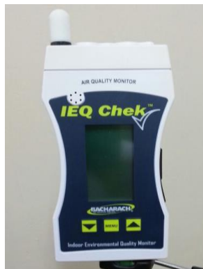
Fig. 3. Contaminant Concentration Device, IEQ Chek
