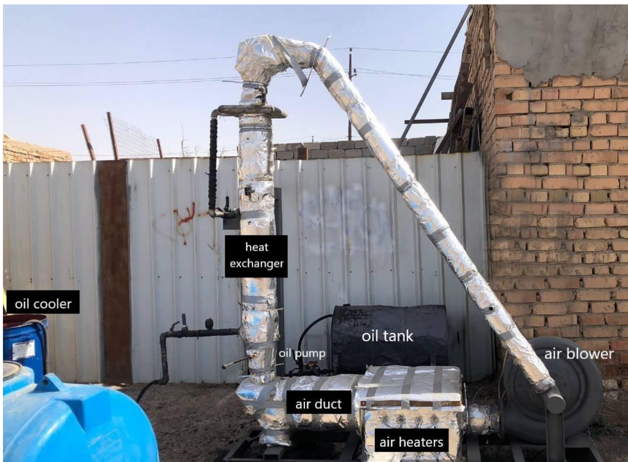
Fig. 2. Illustrated flow diagram of the test rig
