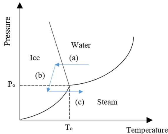
**Fig. 1.** Water Phase Diagram and VFD steps; (a) freezing, (b) vacuum, (c) drying
