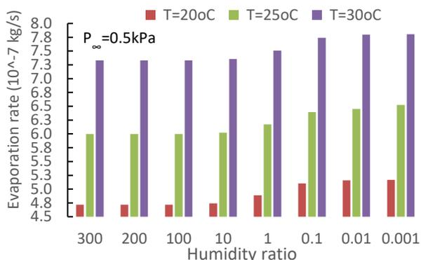
**Fig. 5.** Air humidity ratio vs drying rate at pressure  $P_{\infty}=0.5\text{kPa}$
