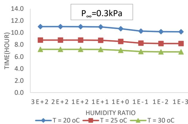
**Fig. 10.** Air humidity ratio vs drying duration at pressure  $P_{\infty}=0.3\text{kPa}$
