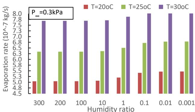
**Fig. 7.** Air humidity ratio vs drying rate at pressure  $P_{\infty}=0.3\text{kPa}$
