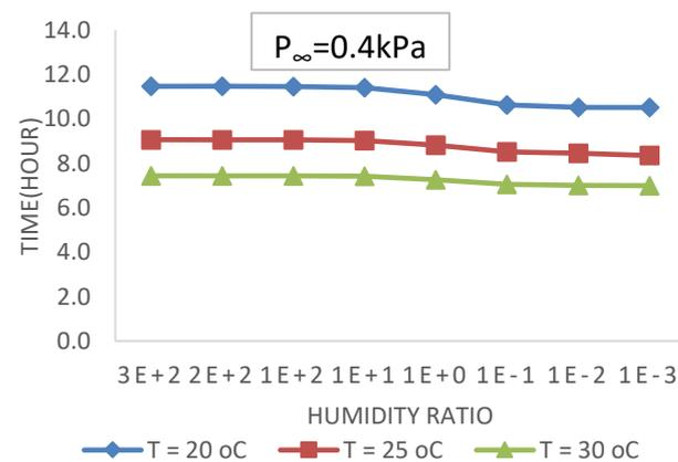
**Fig. 9.** Air humidity ratio vs drying duration at pressure  $P_{\infty}=0.4\text{kPa}$
