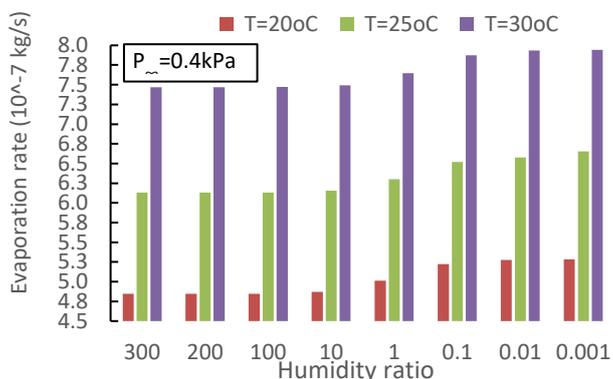
**Fig. 6.** Air humidity ratio vs drying rate at pressure  $P_{\infty}=0.4\text{kPa}$
