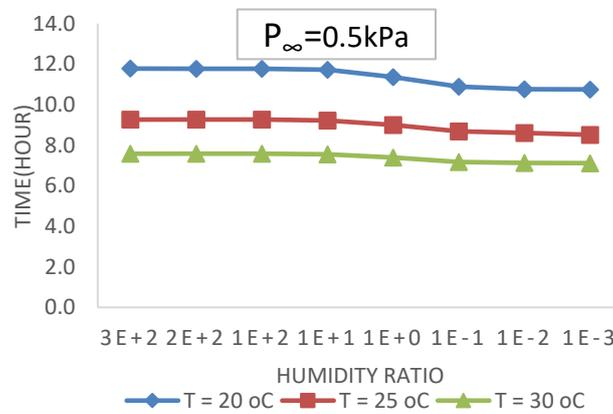
**Fig. 8.** Air humidity ratio vs drying duration at pressure  $P_{\infty}=0.5\text{kPa}$
