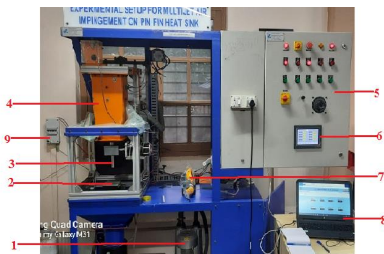
Fig. 1. Experimental system for analysis of steady-state air jet impingement on a heated aluminum plate: 1. inlet blower, 2. target plate assembly, 3. Nozzle, 4. Phelum, 5. control panel, 6. HMI, 7. Thermal infrared camera, 8. DAQ system, 9. Mains Supply
