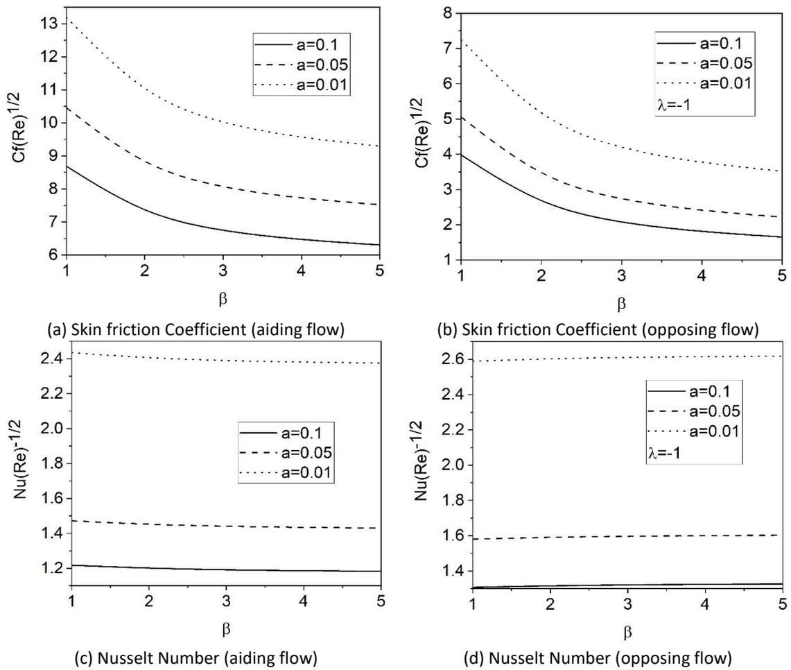
**Fig. 7.** Effect of  $a$  on  $\sqrt{Re}C_f$  and  $\frac{Nu}{\sqrt{Re}}$
