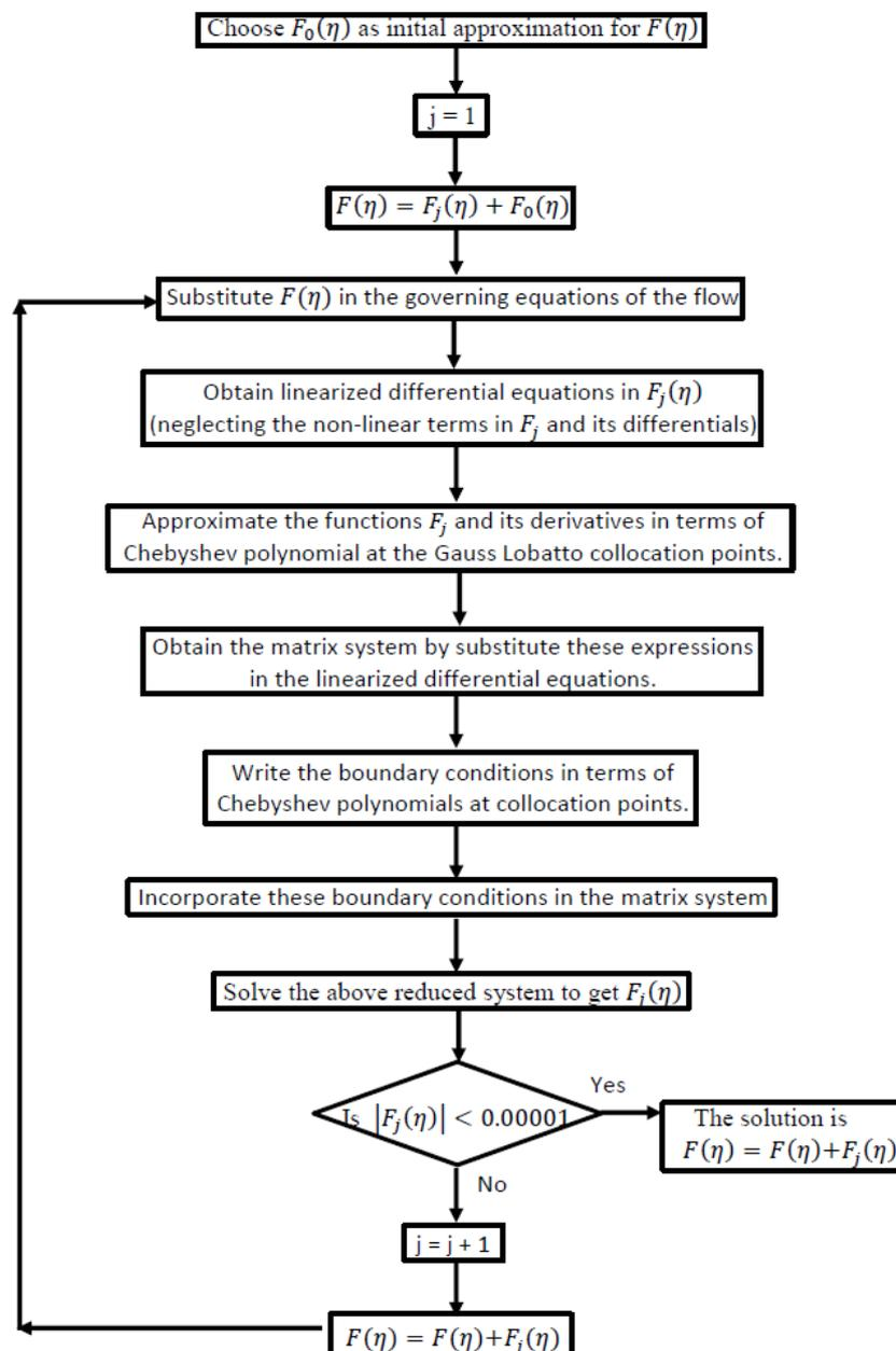
Fig. 2. Flow chart for the solution of the problem
