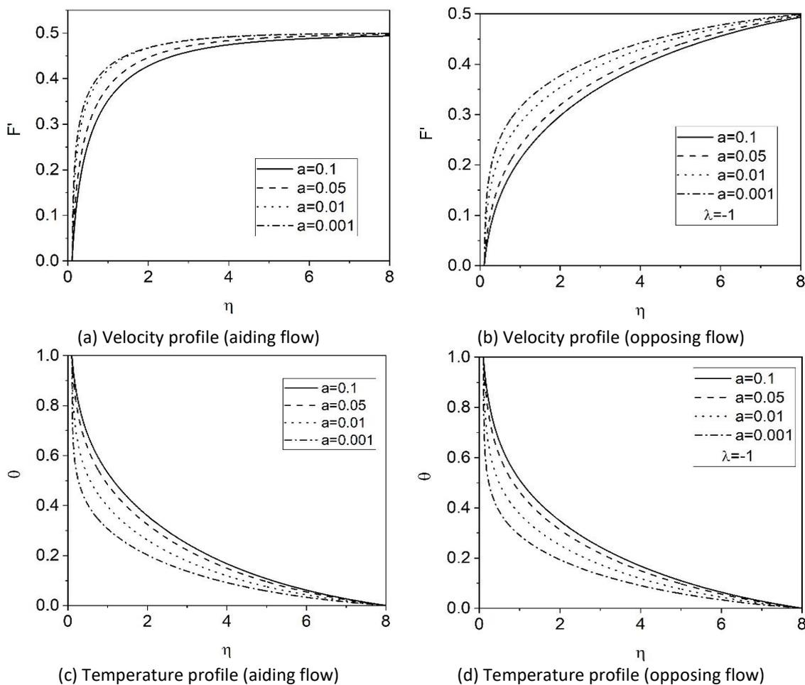
**Fig. 3.** Effect of size of the needle on the velocity and temperature
