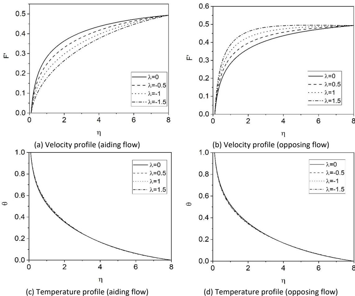
**Fig. 5.** Effect of  $\lambda$  on the velocity and temperature
