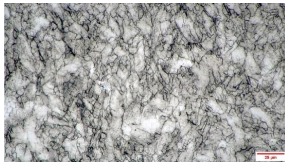
Fig. 4. Microstructure of TNTZ sample before the oxidation process
