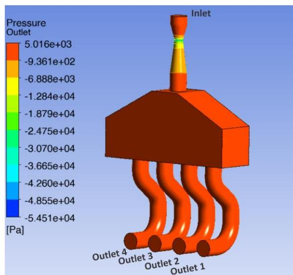
**Fig. 6.** Suggestion-2 (Single plenum; one inlet and four outlet)
