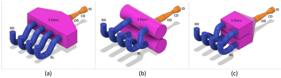
**Fig. 1.** Design of plenum chamber; (a) Single, (b) Dual, and (c) New Geometry
