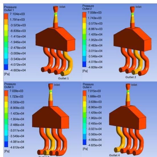
Fig. 5. Suggestion-1 (Pressure distribution in a single plenum design)
