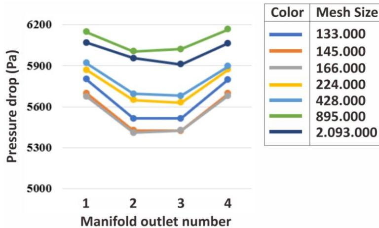
Fig. 4. Pressure drops distribution of independent mesh simulation
