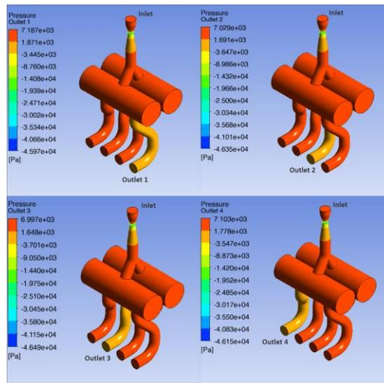
**Fig. 7.** Suggestion-1 (Pressure distribution in dual plenum intake manifold)
