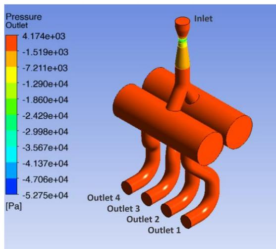
**Fig. 8.** Suggestion-2 (Dual plenum; one inlet and four outlet)
