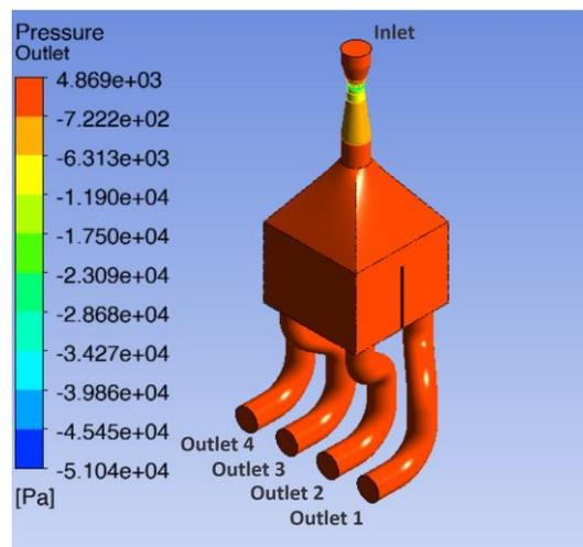
**Fig. 10.** Suggestion-2 (New geometry plenum; one inlet and four outlet)
