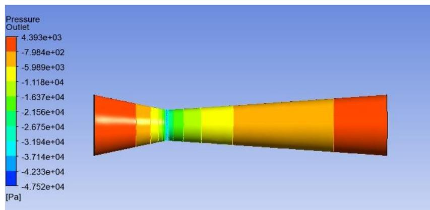
**Fig. 3.** Pressure contours at restrictor region
