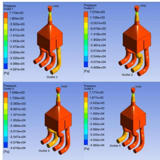
**Fig. 9.** Suggestion-1 (Pressure distribution in intake manifold new geometry)
