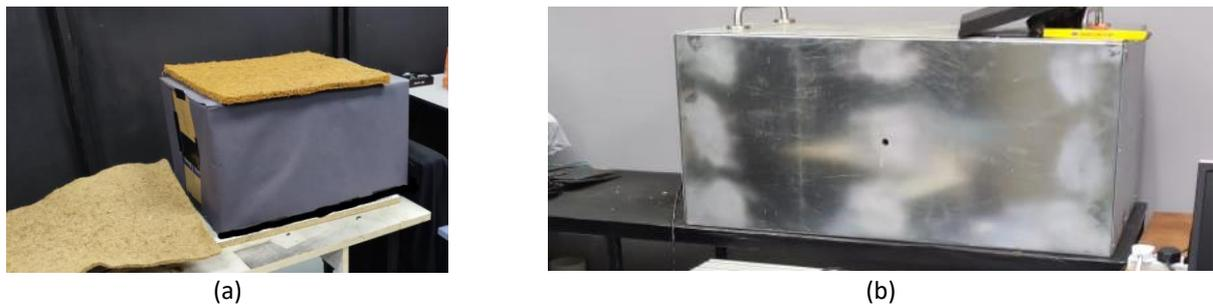
**Fig. 3.** (a) A wooden soundbox with coconut fibre foam and (b) an aluminium box with insulation foam to suppress the noise from the thermoacoustic test rig
