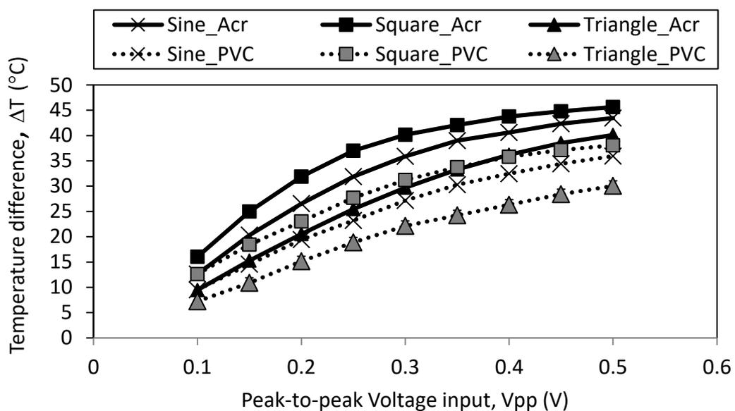
Fig. 5. Temperature difference between the two ends of the stack when different waveforms were tested at various peak-to-peak voltage, Vpp input
