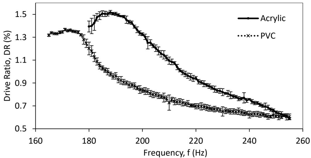
Fig. 4. Resonance frequency test for thermoacoustic rest rig with two different materials
