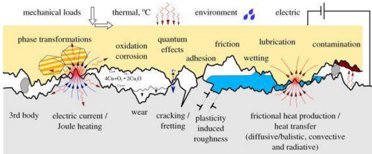
**Fig. 2.** Illustrations for tribological phenomena multiphysical nature in which two solids having coarse surfaces and related microstructural material are having contact and exposure to variety of loads: electrical, thermal, environmental and mechanical [7]
