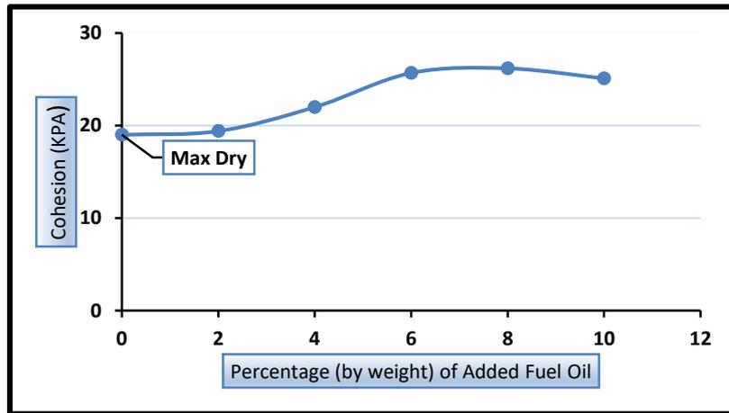
Fig. 5. The Effect of Fuel Oil on Cohesion
