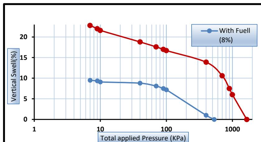
Fig. 8. The Effect of (8% by weight) Added Fuel Oil on the Relationship of Vertical Swell (%) - Applied Pressure
