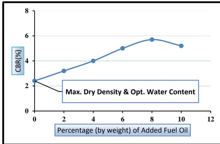
**Fig. 3.** The Effect of Fuel Oil on CBR
