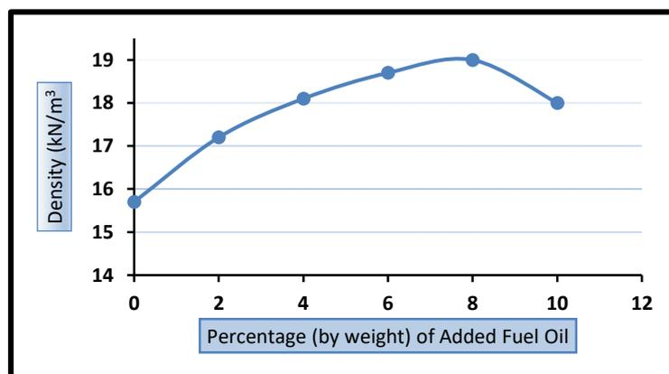
**Fig. 2.** The Effect of Fuel Oil on Dry Density
