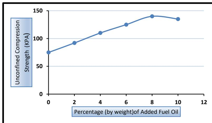
**Fig. 4.** The Effect of Fuel Oil on Unconfined Compression Strength
