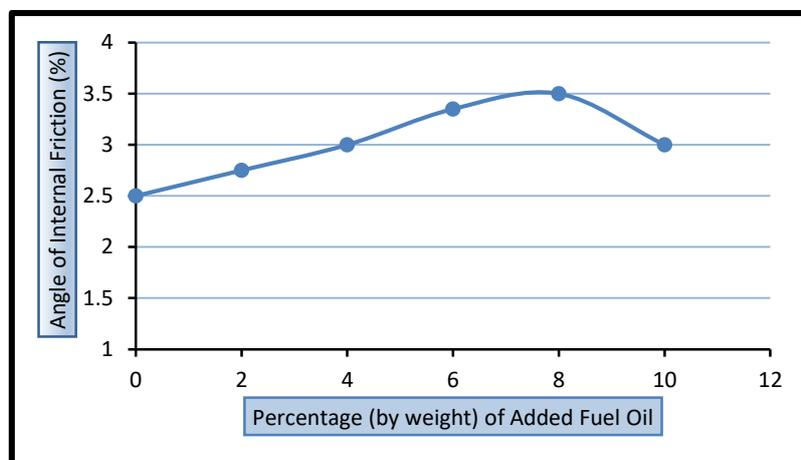
Fig. 6. The Effect of Fuel Oil on Angle of Internal Friction
