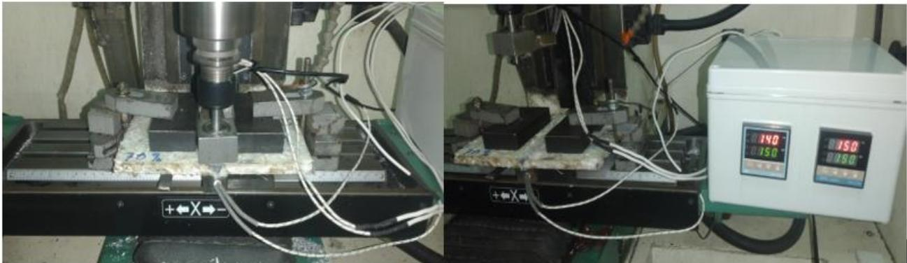
**Fig. 1.** The process of welding short fiberglass-HDPE composite specimens with controlled temperature, feeding, and speed using an NC Milling machine and at the same time being formed into tensile test specimens according to ASTM D3039 to determine the mechanical properties of the joint
