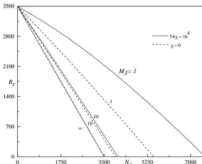
**Fig. 6.** Variation of  $R_c$  versus  $N_c$  for different  $M_3$  and  $\chi$  for  $\delta = 0.02$ ,  $\sigma^2 = 50$  and  $Bi = 2$
