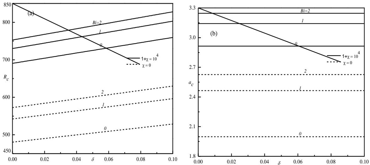
**Fig. 2.** Variation of (a)  $R_c$  and (b)  $a_c$  with  $\delta$  for different  $Bi$  and  $\chi$  for  $M_3 = 1$ ,  $M_1 = 5$  and  $\sigma^2 = 50$
