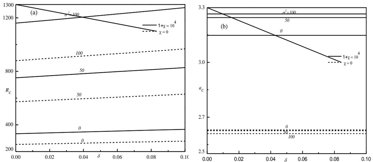
**Fig. 3.** Variation of (a)  $R_c$  and (b)  $a_c$  with  $\delta$  for different values of  $\sigma^2$  and  $\chi$  for  $M_3 = 1$ ,  $M_1 = 5$ ,  $Bi = 2$
