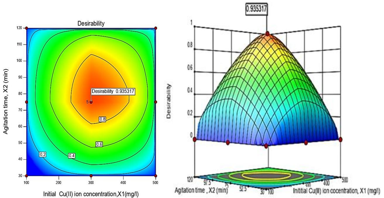
**Fig. 4.** Optimization Response surface contour and 3-D for desirability ramp plots for the effect initial Cu(II) ions concentration and agitation time (min) on Cu(II) removal (mg/L)
