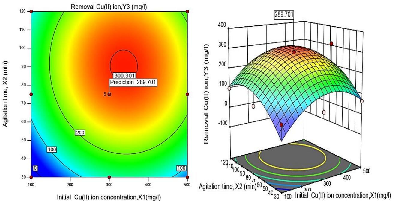
**Fig. 3.** The PB response surface contour and 3-D plots for the effect of initial Cu(II) ions concentration and agitation time (min) on Cu(II) removal (mg/L)
