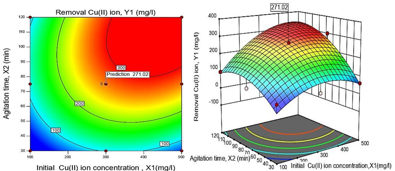
**Fig. 1.** The NB response surface contour and 3-D plots for the effect of initial Cu(II) ions concentration and agitation time (min) on Cu(II) removal (mg/L)
