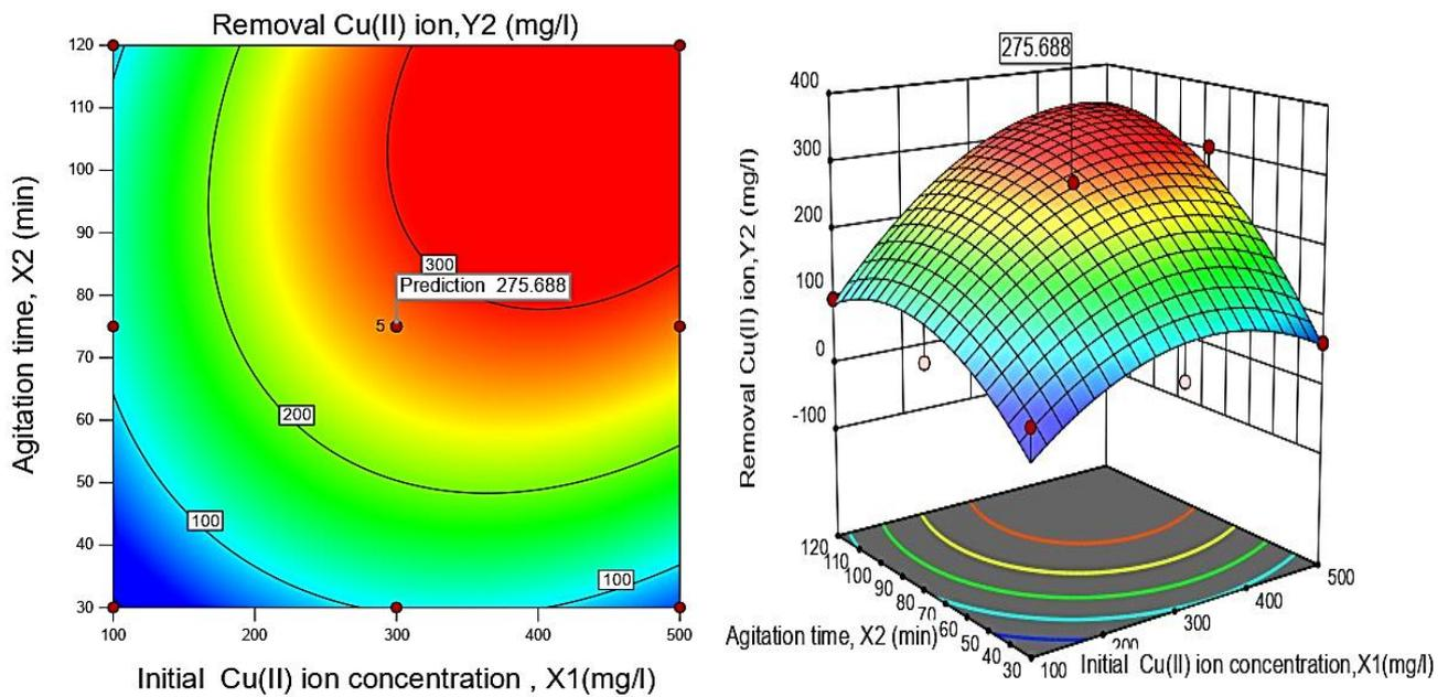
**Fig. 2.** The IB response surface contour and 3-D plots for the effect initial Cu(II) ions concentration and agitation time (min) on Cu(II) removal (mg/L)
