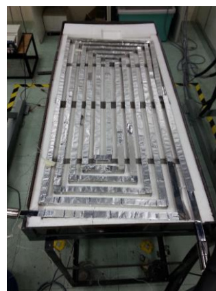
Fig. 2. Spiral absorber attached to the back of the PV
