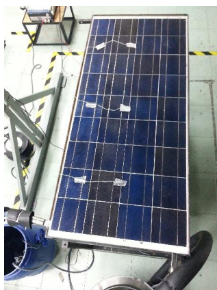
Fig. 1. PVT water collector under a solar simulator
