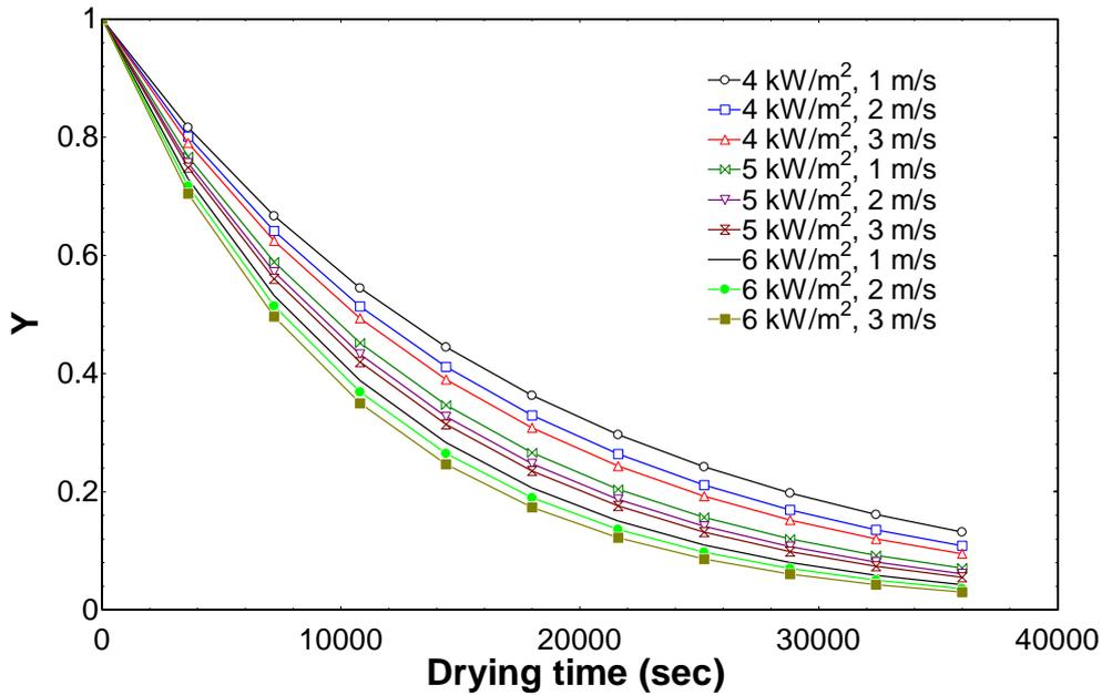
Fig. 2. Drying curves under various drying conditions
