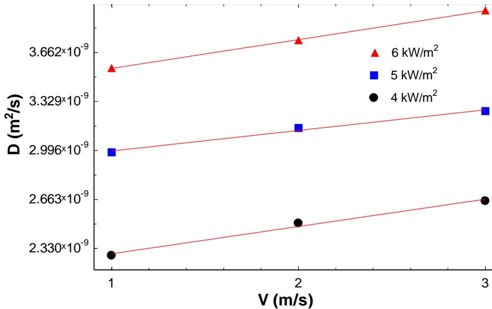
Fig. 3. Variation of moisture diffusivity with drying conditions
