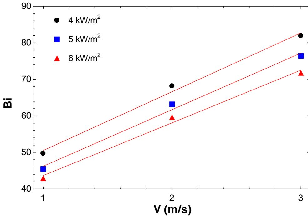
Fig. 5. Observed Biot number at different drying conditions
