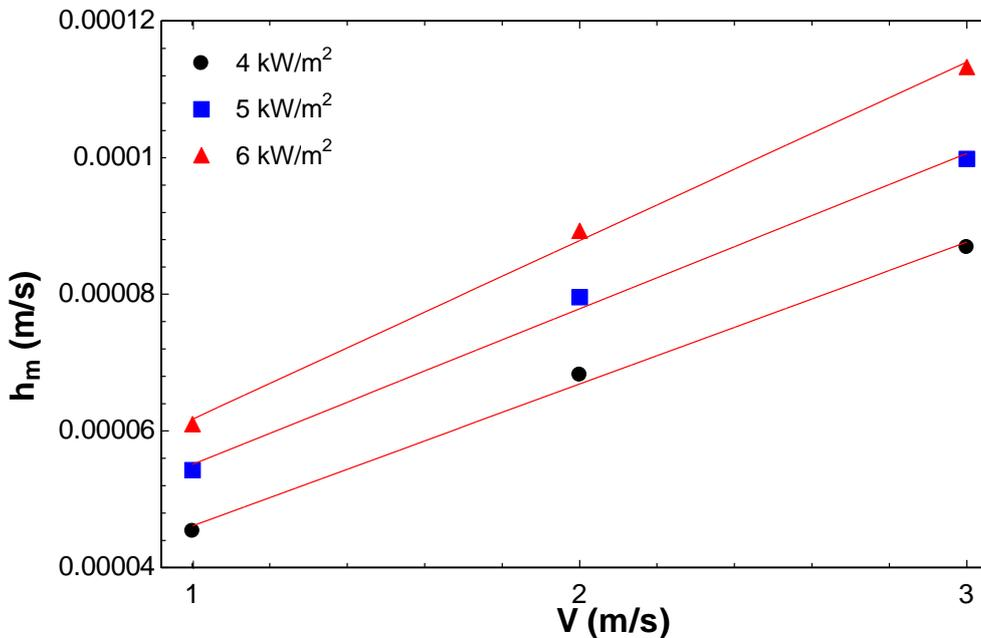
Fig. 4. Variation of moisture transfer coefficient with drying conditions
