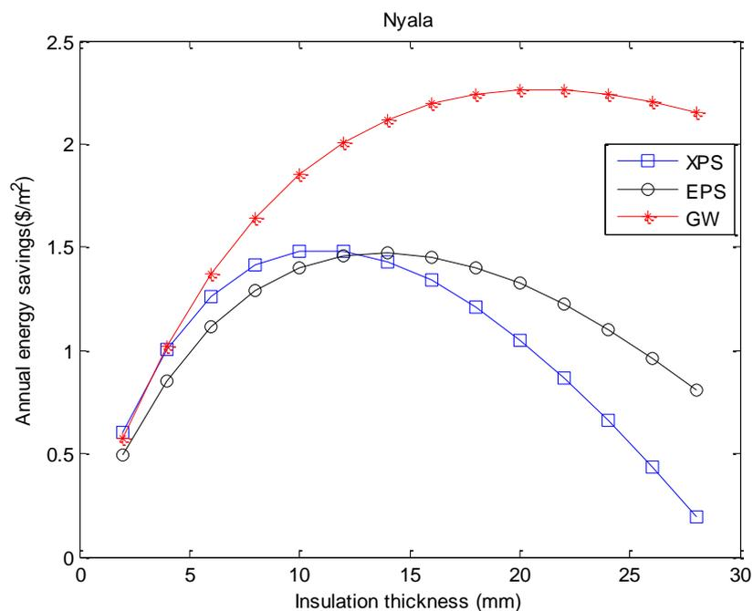
**Fig. 9.** Comparison of the annual energy savings of all insulation materials in the case of the cooling requirement for selected fired clay bricks in Nyala
