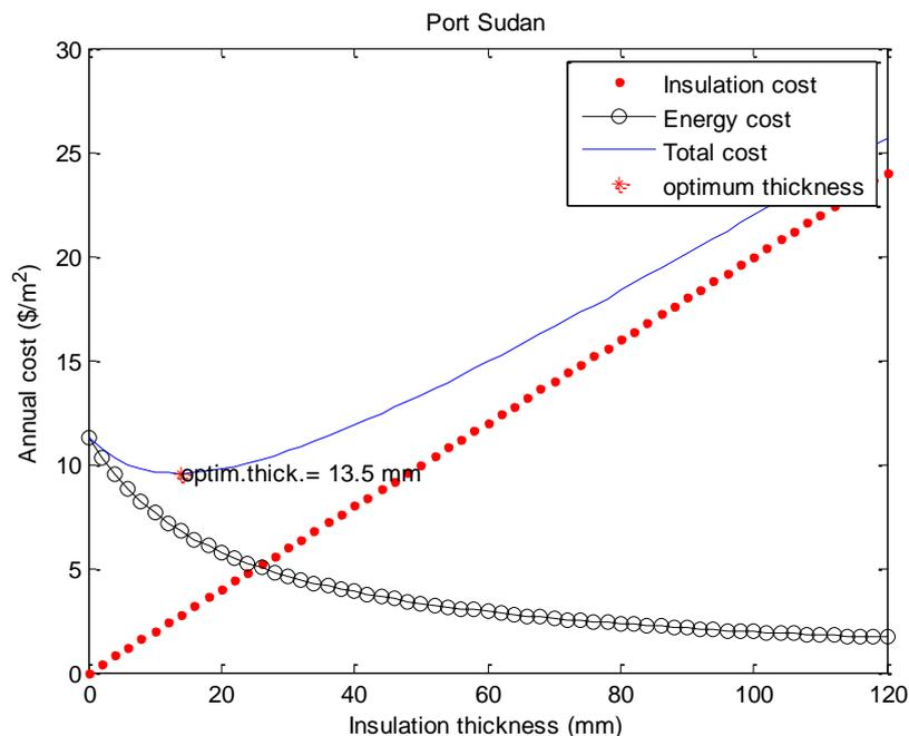
**Fig. 4.** Effect of the insulation thickness of extruded polystyrene (XPS) on the total cost in case cooling energy requirement used perforated red brick in Port Sudan
