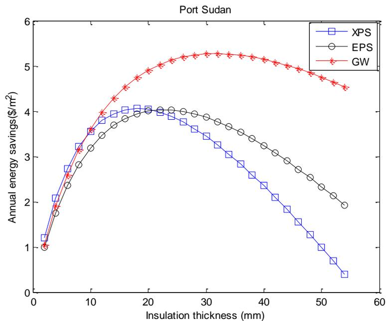
**Fig. 8.** Comparison of the annual energy savings of all insulation materials in the case of the cooling requirement for selected fired clay bricks in Port Sudan
