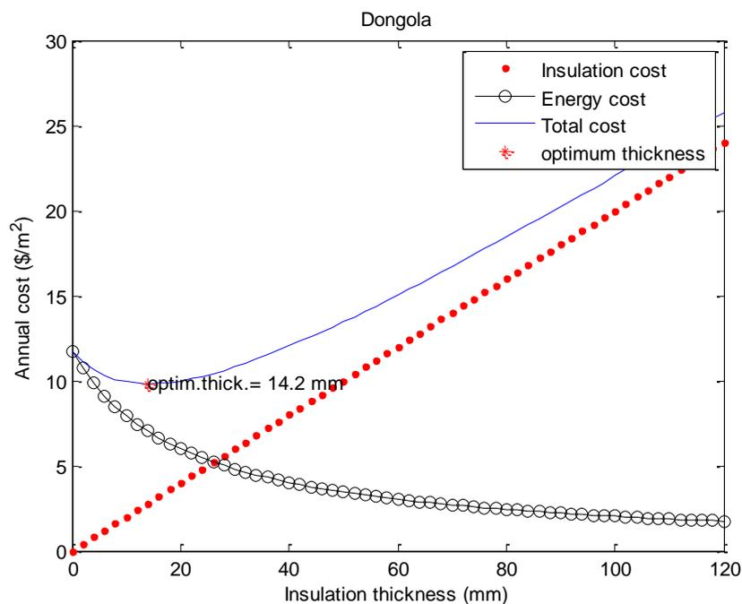
**Fig. 3.** Effect of the insulation thickness of extruded polystyrene (XPS) on the total cost in case cooling energy requirement used perforated red brick in Dongola
