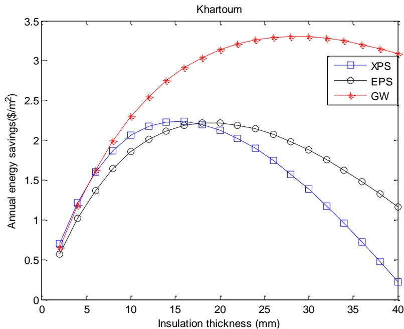
**Fig. 6.** Comparison of the annual energy savings of all insulation materials in the case of the cooling requirement for selected fired clay bricks in Khartoum
