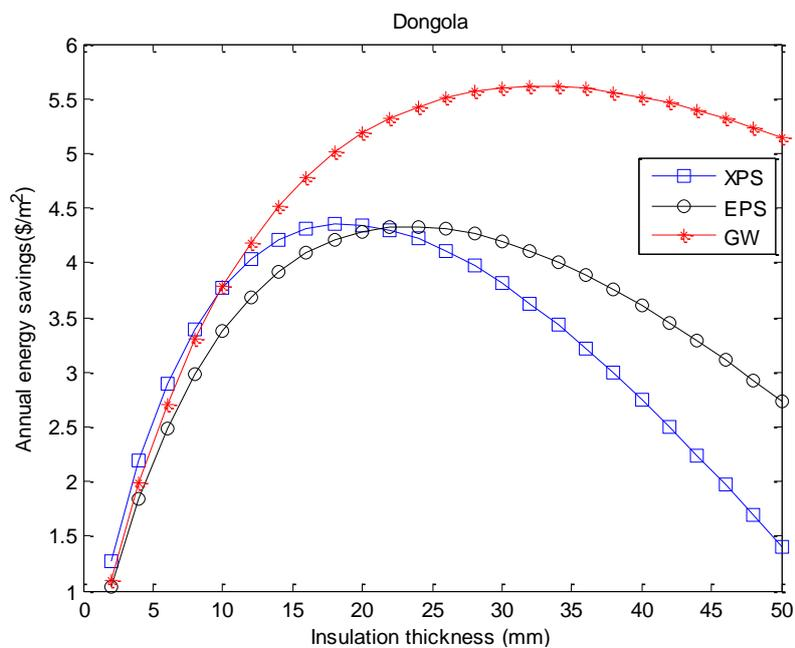
**Fig. 7.** Comparison of the annual energy savings of all insulation materials in the case of the cooling requirement for selected fired clay bricks in Dongola
