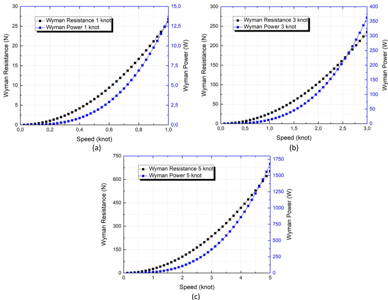
**Fig. 7.** Graph of Wyman resistance and Wyman power of the boat; (a) 1 knot, (b) 3 knot, and (c) 5 knot
