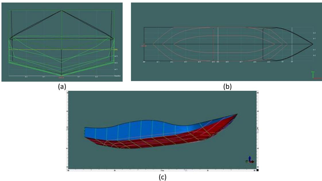
**Fig. 3.** Pakura boat design on maxsurf software; (a) body plan, (b) plan, (c) perspective
