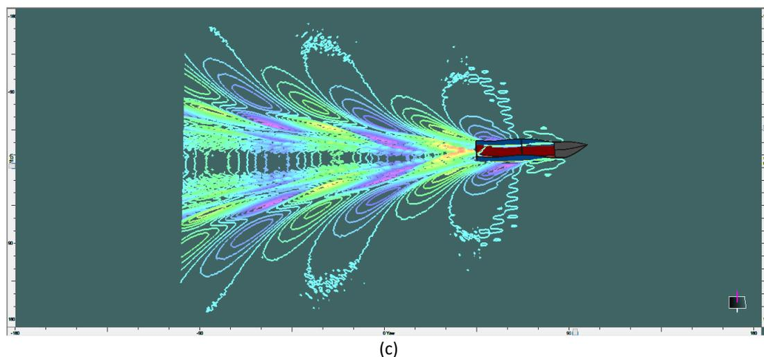
Fig. 6. Sea wave profile when the boat is operating; (a) 1 knot, (b) 3 knots, and (c) 5 knots
