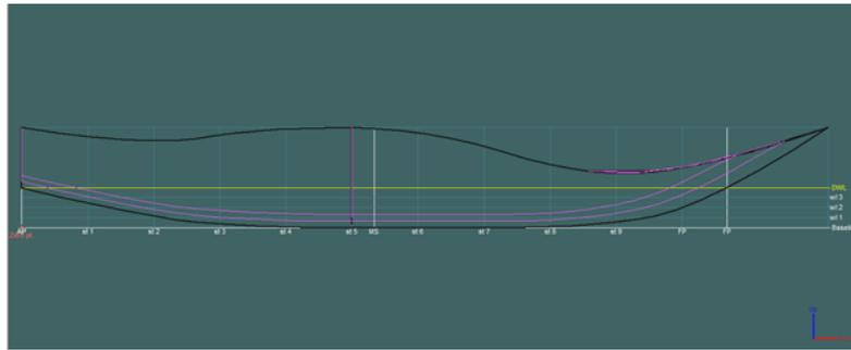
**Fig. 2.** Baseline pakura boat design on maxsurf software
