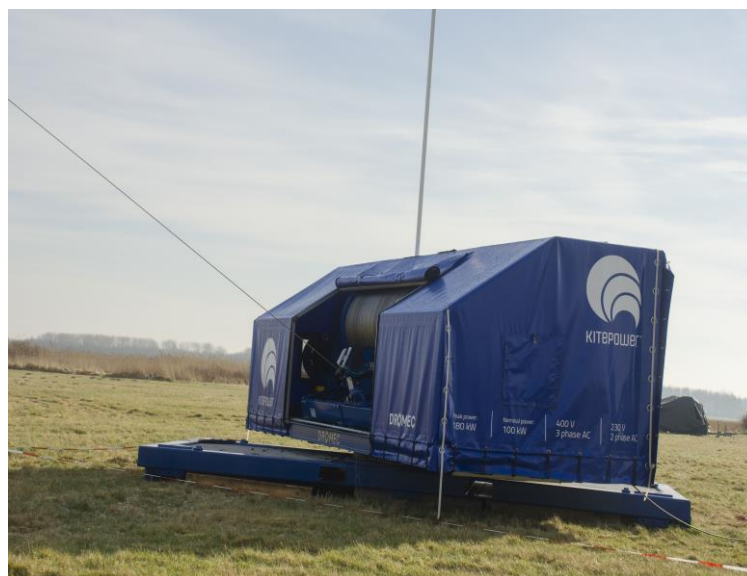
Fig. 2. The power train of kite power system [5]
