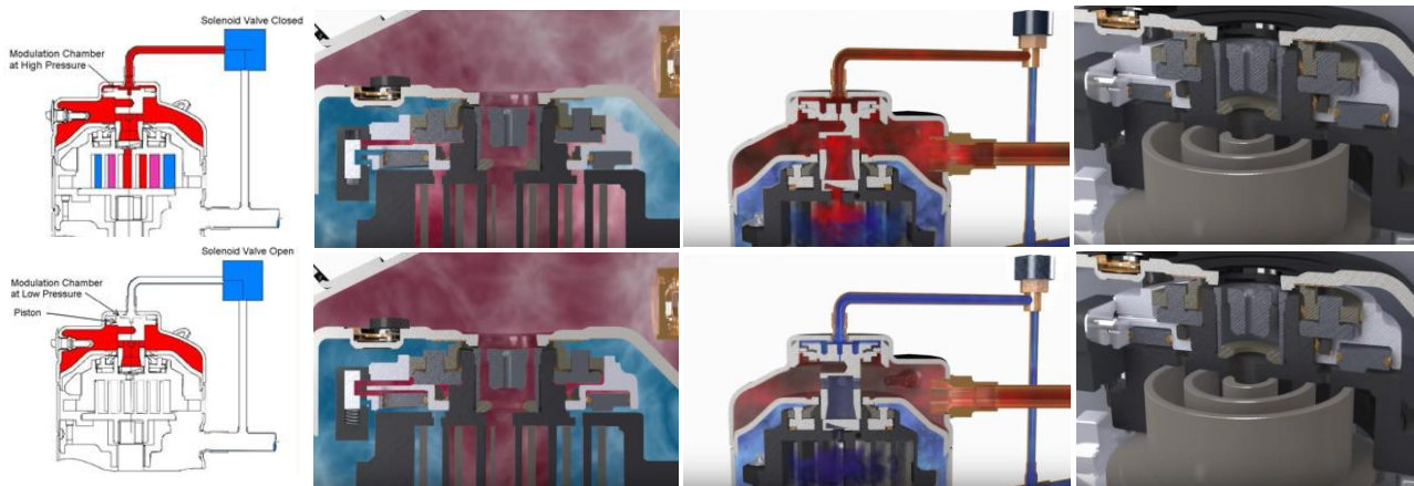
Fig. 4. How digital scroll compressor operated
