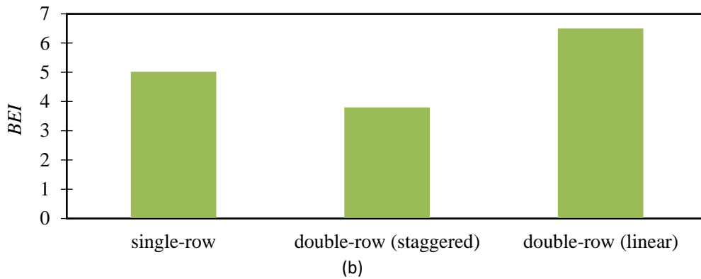
Fig. 32. The windbreak arrangements of the (a) shelter effect under an incoming velocity of U_{ref} = 8.46 m/s, and (b) BEI for different rows
