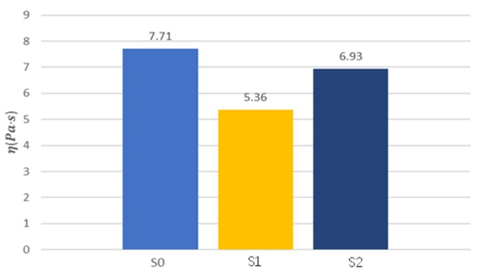
Fig. 4. Plastic viscosity of CPB of different cementing materials
