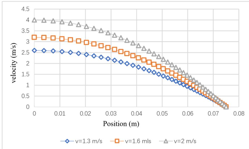
**Fig. 7.** The cross-sectional velocity distribution in the pipe under different velocity
