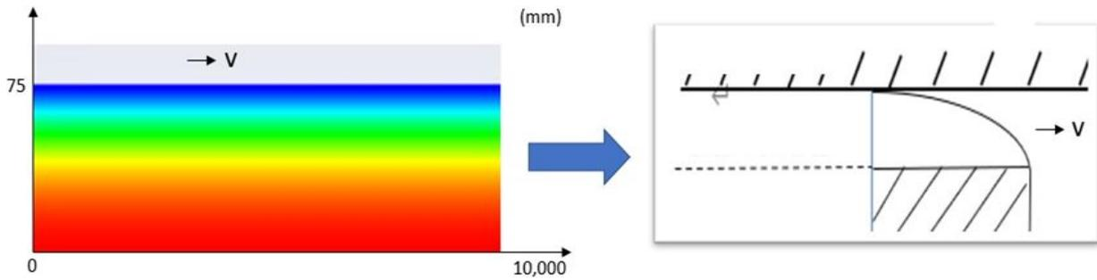
**Fig. 6.** Flow pattern of CPB slurry in pipeline
