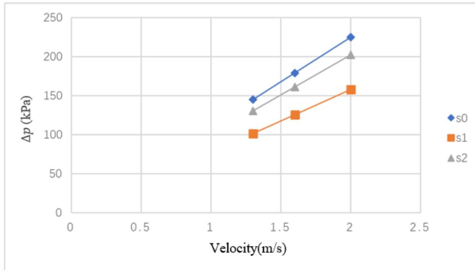
**Fig. 8.** Pressure loss of CPB slurry with different cementing materials during transportation
