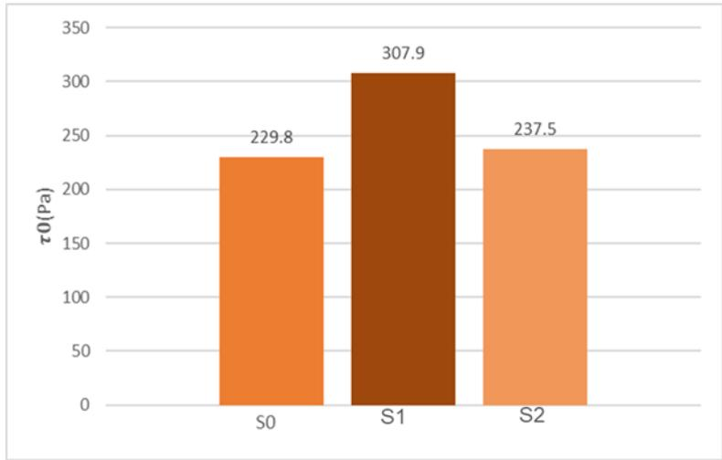
Fig. 5. Yield stress of CPB of different cementing materials
