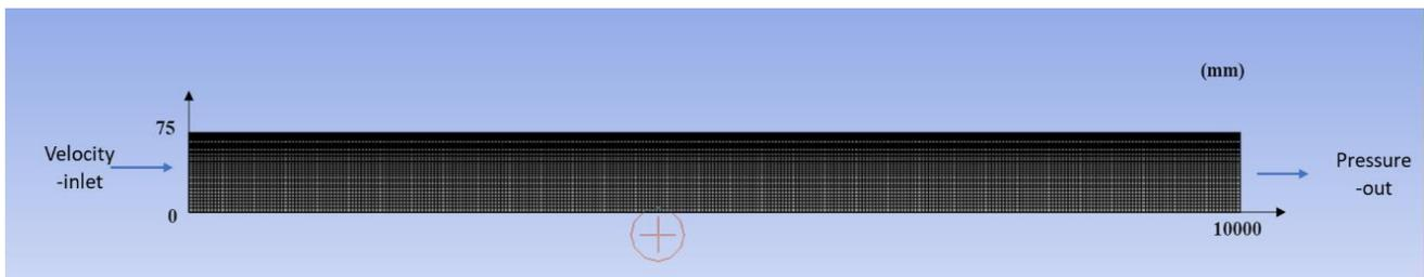
**Fig. 2.** The grid and size of pipe model
