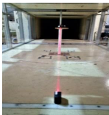
Fig. 11. Use of the Laser Light Device to align the model inside the section test of the wind tunnel
