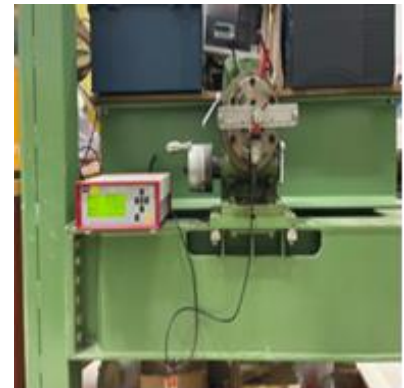
Fig. 15. Calibration set-up of the torque sensor
