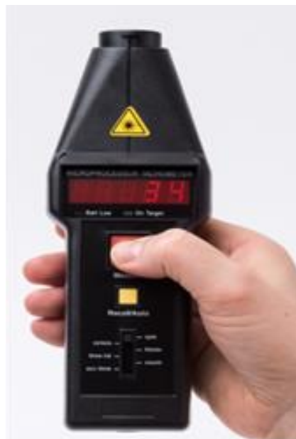
Fig. 17. Tachometer to measure the rotor blade rpm
