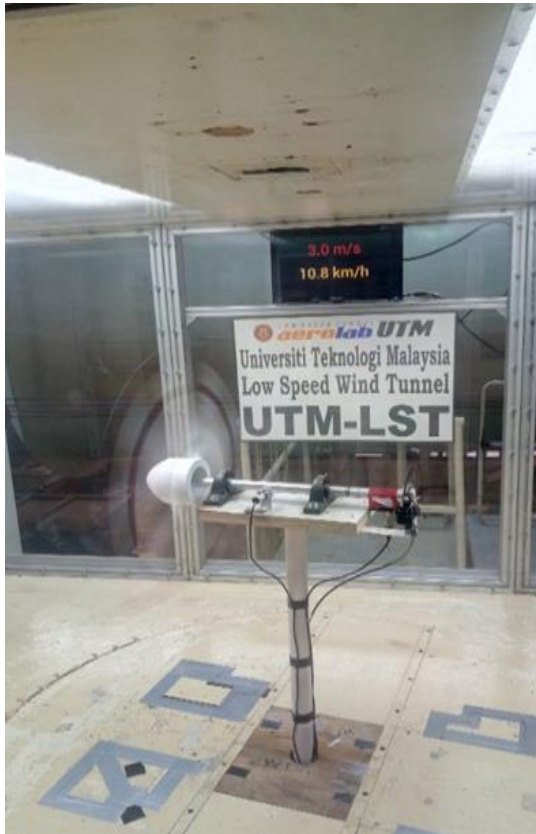
Fig. 6. The two-airfoil turbine inside the section testing of the UTM-LST wind tunnel
