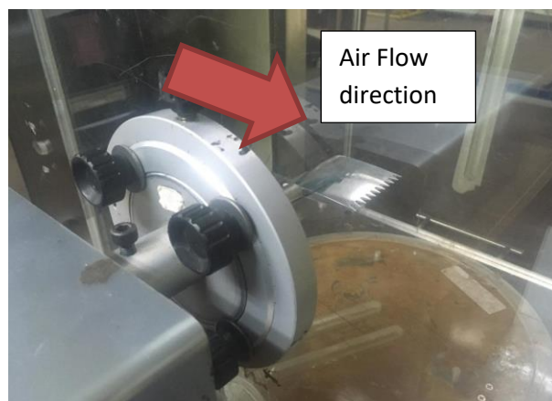
Fig. 4. Side view of wing model in the wind tunnel
