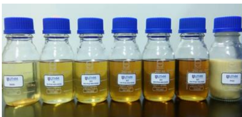
Fig. 2. Biofuel from Mixing of PFAD and Diesel
