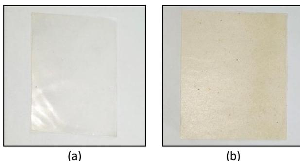
Fig. 2. (a) PC-biofilm and (b) WS-biofilm
