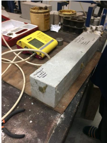
Fig. 1. Ultrasonic pulse velocity test
