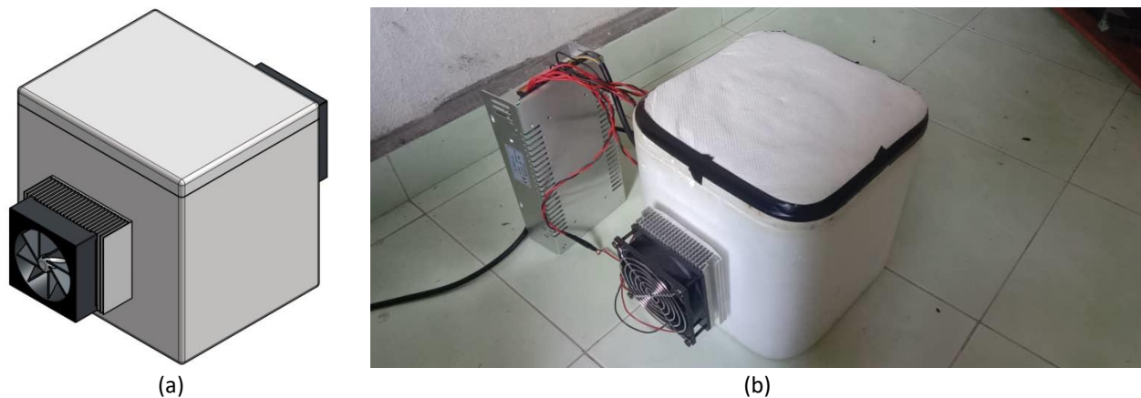
Fig. 2. Peltier-Based Thermoelectric (a) Cooling Box Final Technical Drawing Design (b) Cooling Box Final Product Result
